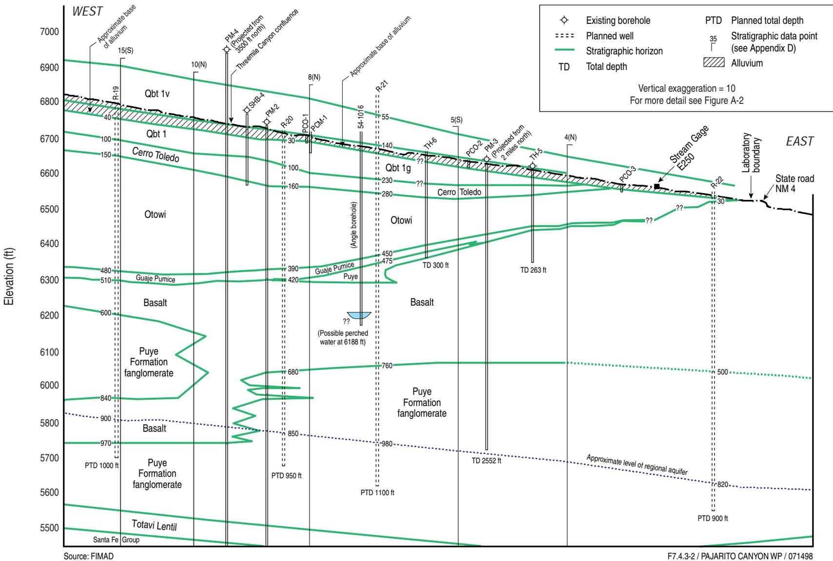
Figure 7.4.3-2. Projected stratigraphic sections for planned regional aquifer wells in lower Pajarito Canyon.
