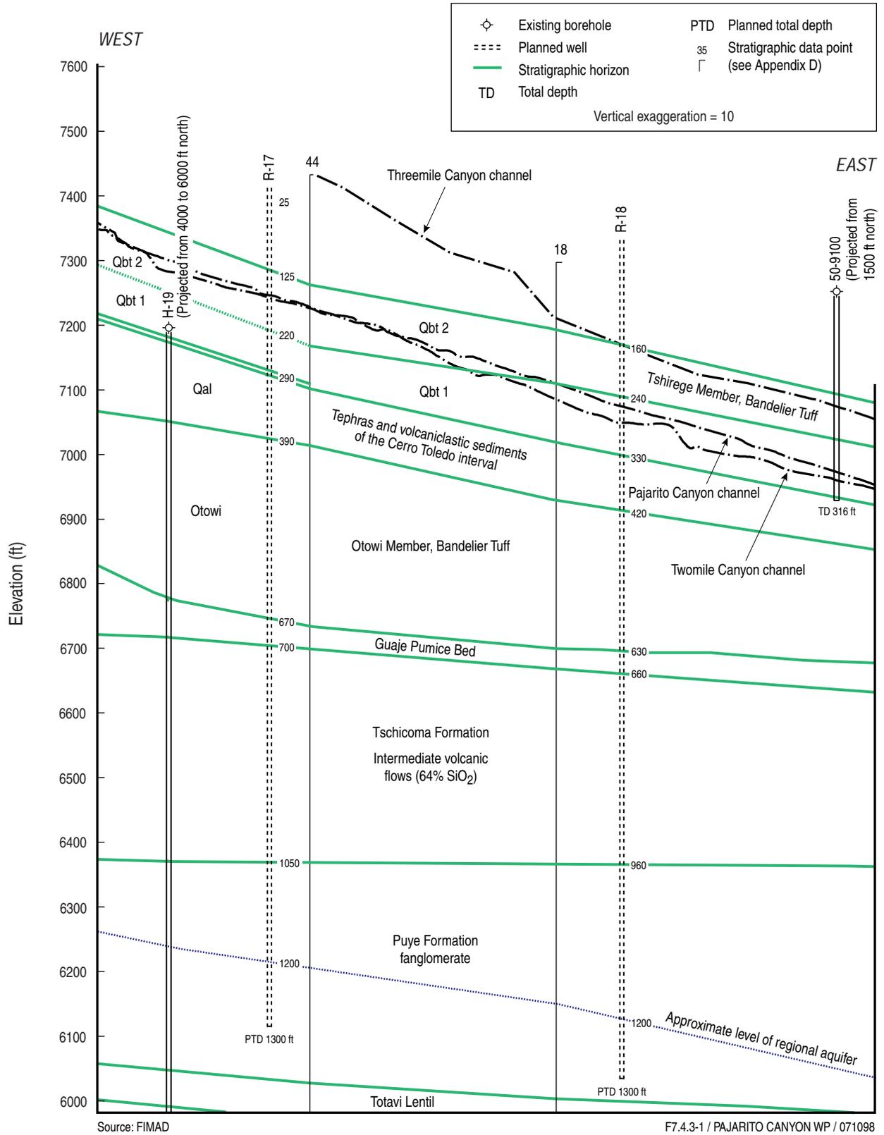
**Figure 7.4.3-1. Projected stratigraphic sections for planned regional aquifer wells in upper Pajarito Canyon.**
