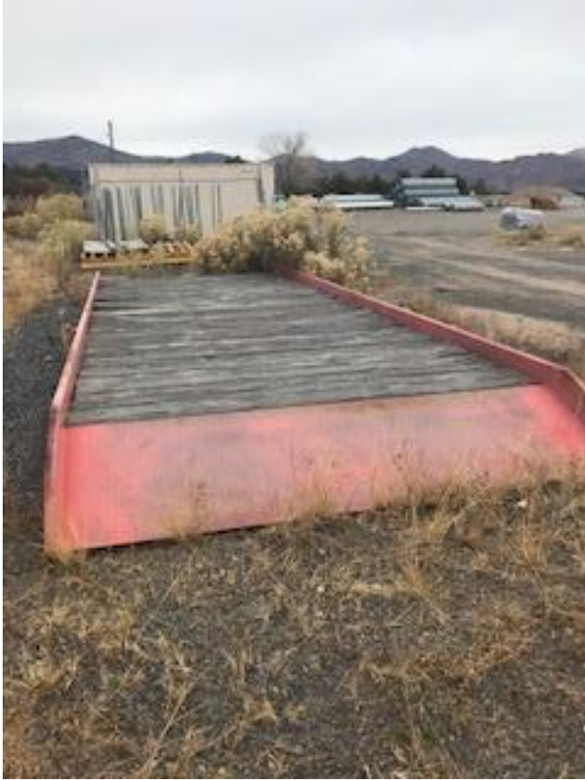
Photo 7. 10-ft X 30-ft pre-fabricated bridge.
