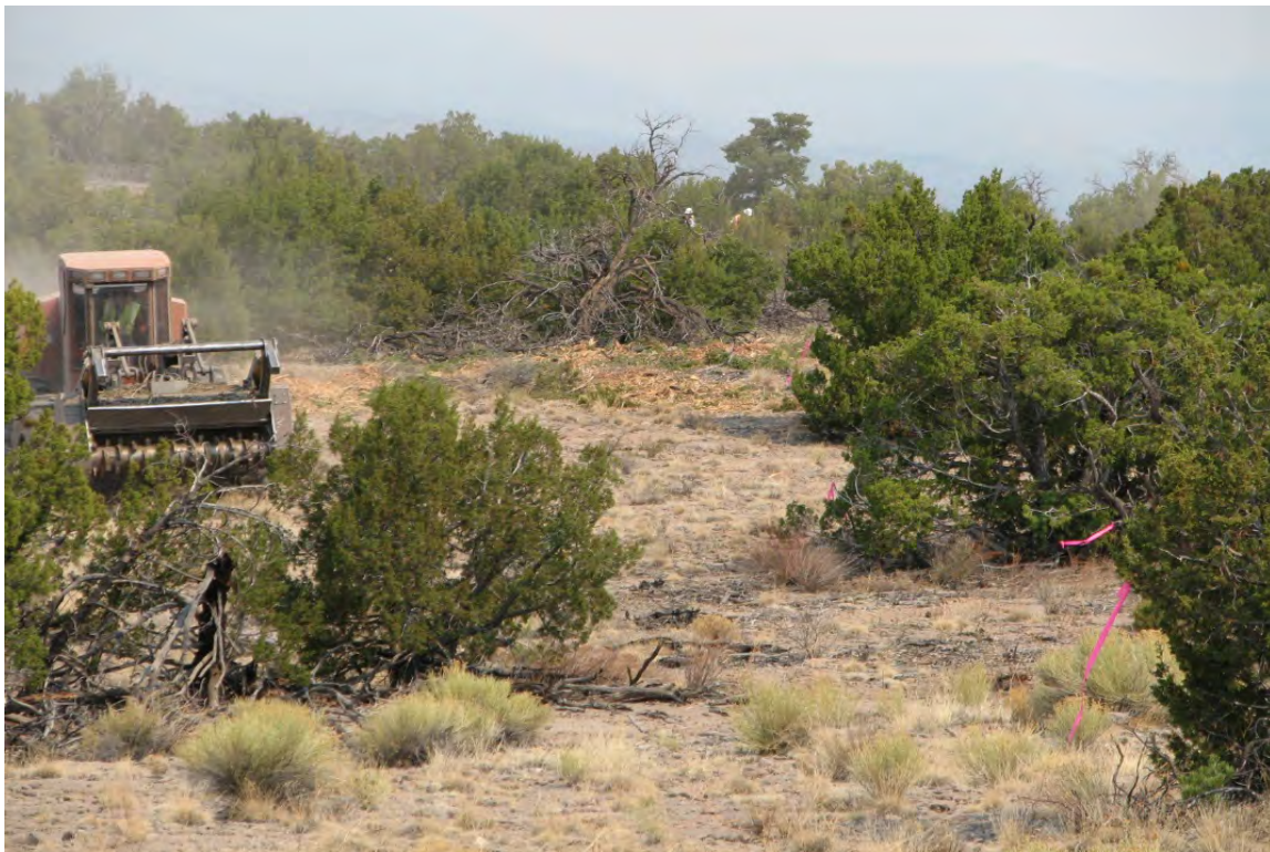
Figure 23.4 Masticator clearing a fire break near an archaeological site during the Las Conchas fire
