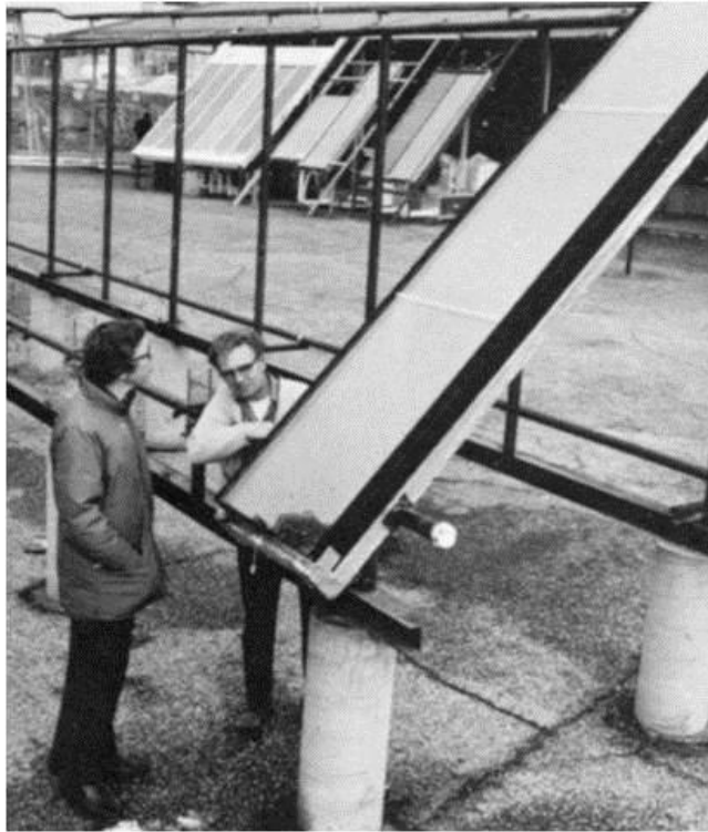
Laboratory scientists examine the first of 40 solar collectors being installed at a test station in 1975 (LASL 1975).
