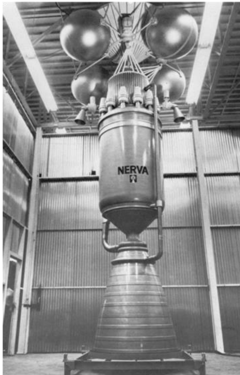
The Project Rover nuclear reactor (photo at left) was designed to power rockets. Compressed hydrogen in the spheres at the top flowed through the reactor core (center) and formed a jet as it exited the nozzle at the bottom (LANL 1983). The Laboratory's Kiwi B-4D reactor (photo at right) being readied for a "hot run" in May 1964 (LASL 1964).
