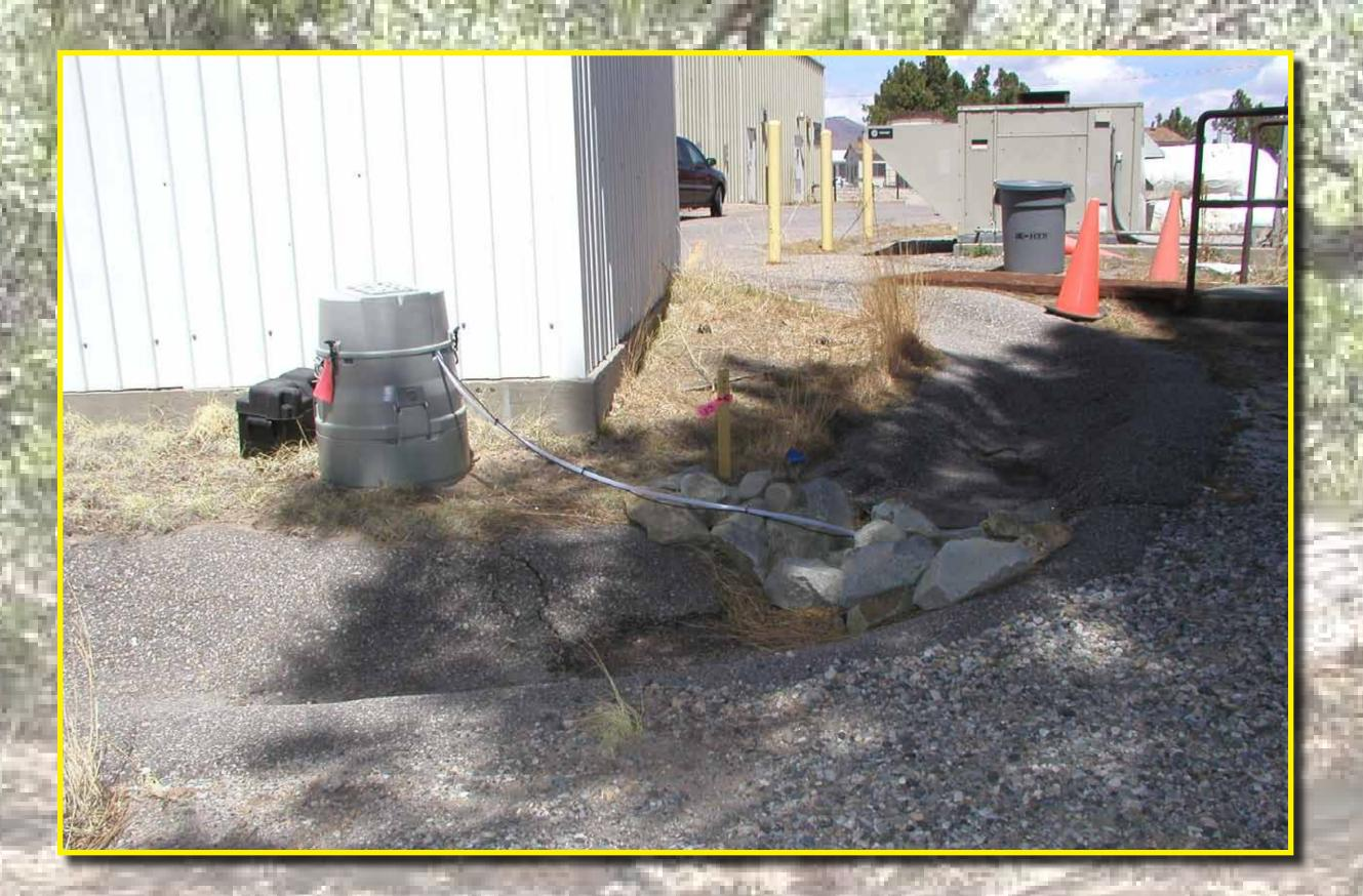
Battery-powered automated samplers are used to collect stormwater samples during runoff events. Sensors turn the sampler on when flow is detected and pump water into bottles located inside the sampler housing. The samplers record the date and time the sample was collected.
