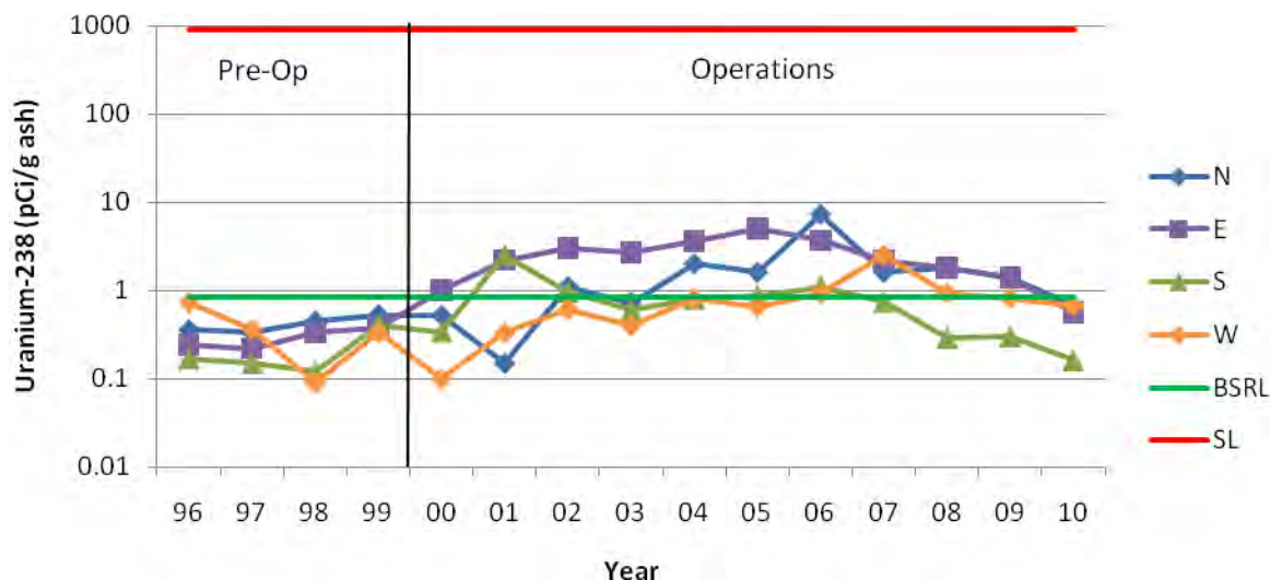
Figure 4. Uranium-238 in overstory vegetation collected from the north (N), east (E), south (S), and west (W) side of the DARHT facility at TA-15 from 1996–1999 (pre-operations) through 2000–2010 (during operations) compared with the baseline statistical reference level (BSRL) and the screening level (SL). Note the logarithmic scale on the vertical axis.
