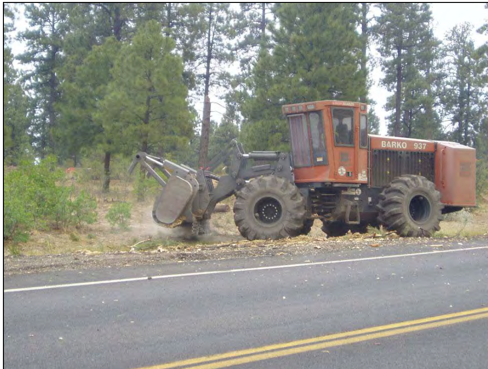
Photograph 17. A masticator works to complete tree thinning along the LANL perimeter.
