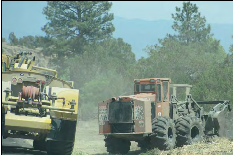
Photograph 19. Preparing a fire line along SR 4 during the Las Conchas fire.
