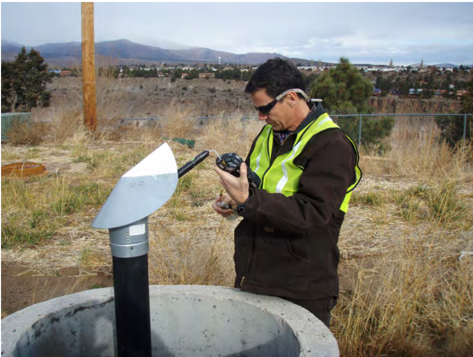
Figure 17 Gas survey at vent riser with spinner
