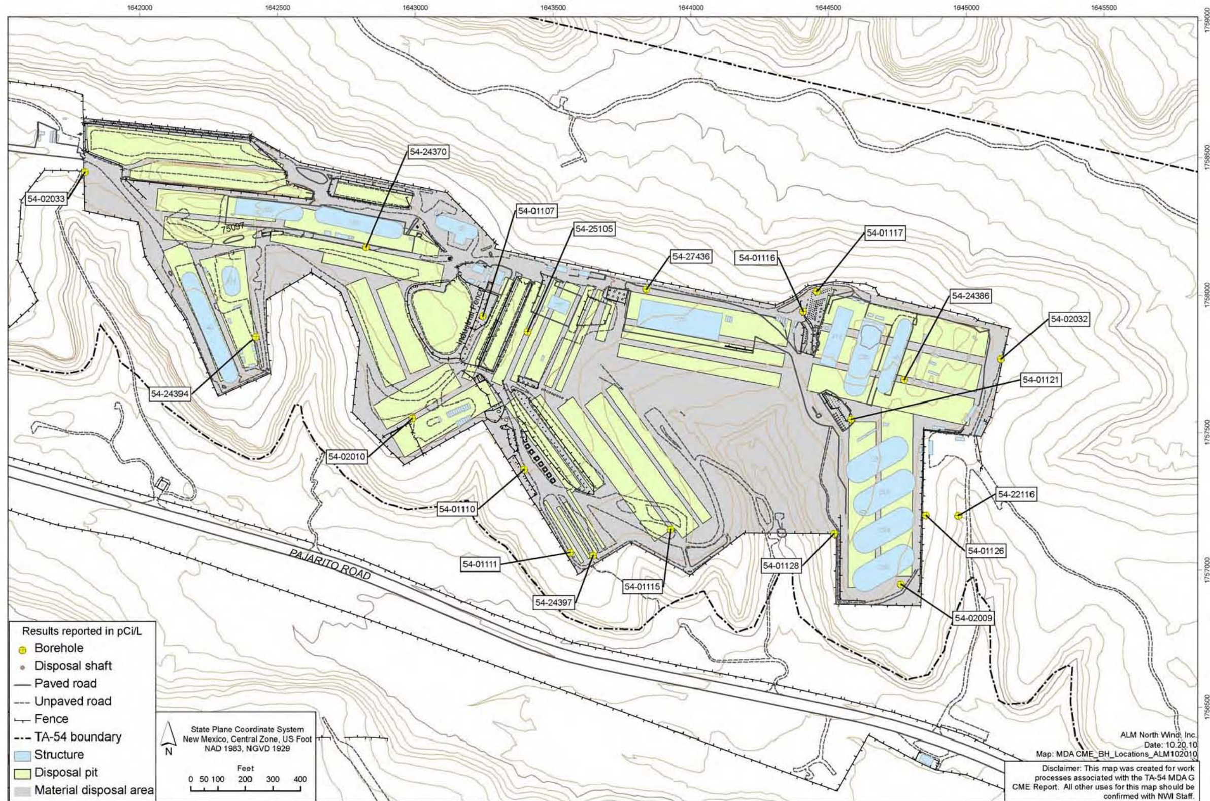
Figure 2.4-4 MDA G pore-gas monitoring borehole locations
