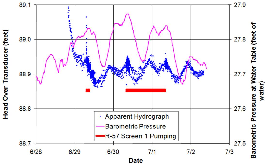
Figure C-7.0-2 Well R-57 screen 2 apparent hydrograph during screen 1 test
