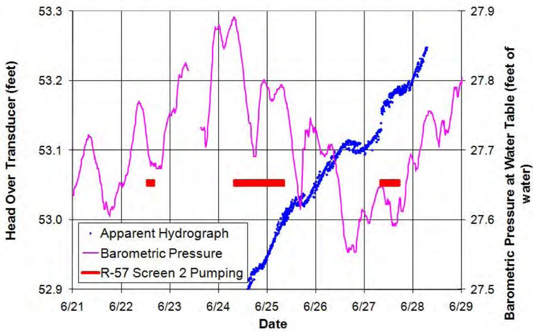
Figure C-7.0-4 Well R-57 screen 1 apparent hydrograph during screen 2 test
