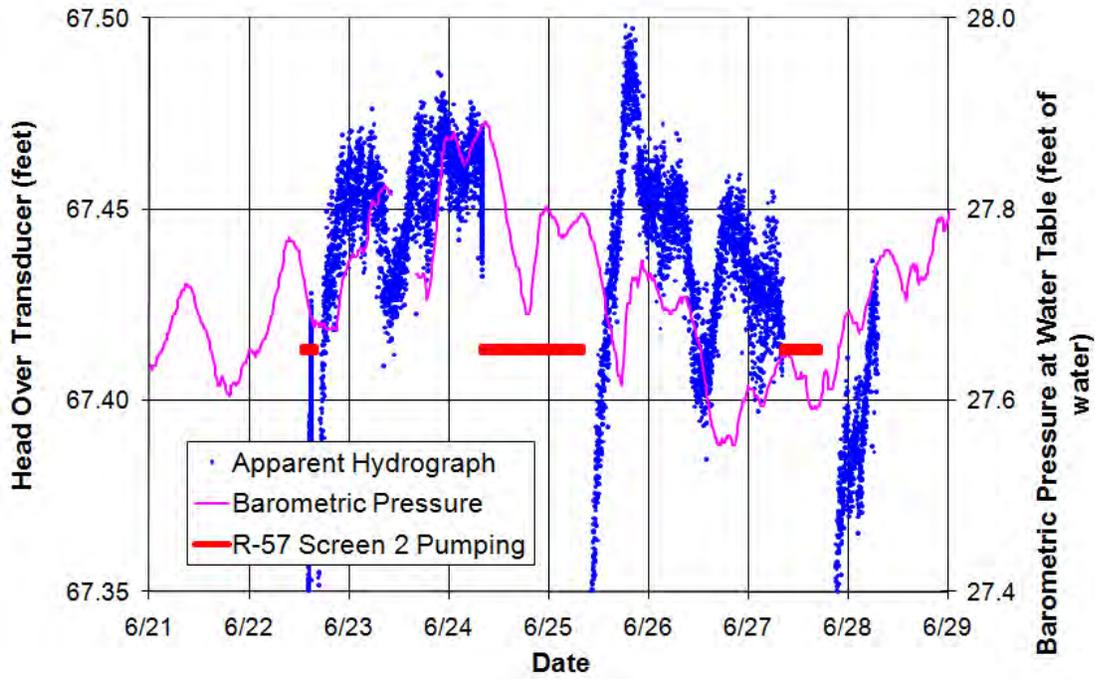
Figure C-7.0-7 Well R-57 screen 2 apparent hydrograph during screen 2 test – expanded scale
