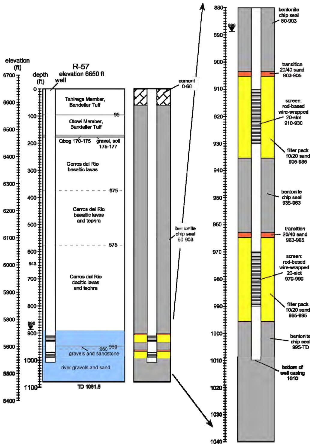
Figure F-2.0-1 Proposed well design for R-57
