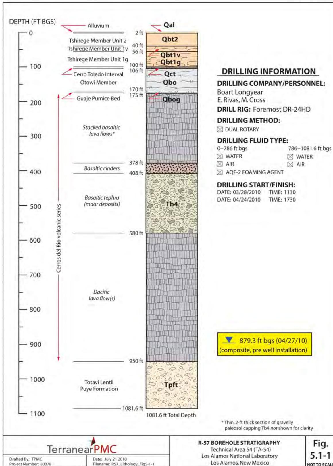
Figure 5.1-1 Monitoring well R-57 borehole stratigraphy
