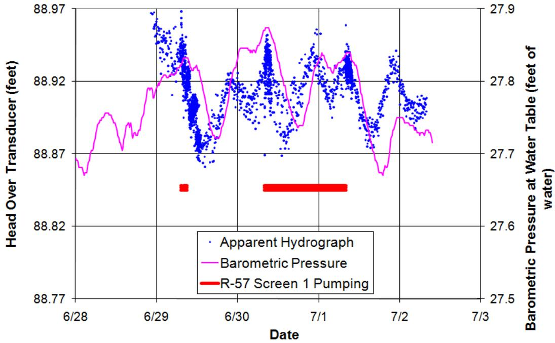
Figure C-7.0-3 Well R-57 screen 2 apparent hydrograph during screen 1 test – expanded scale
