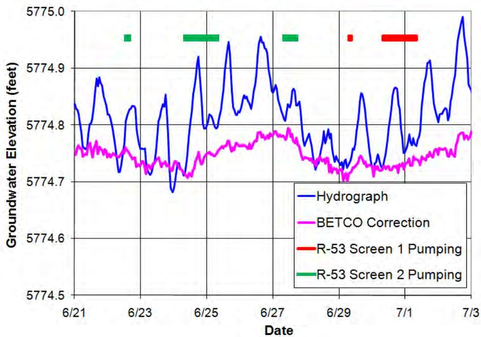
Figure C-7.0-10 Well R-49 screen 1 hydrograph
