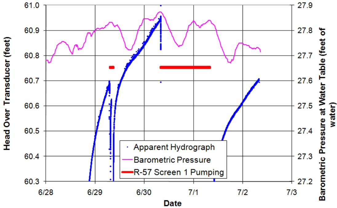
Figure C-7.0-1 Well R-57 screen 1 apparent hydrograph during screen 1 test
