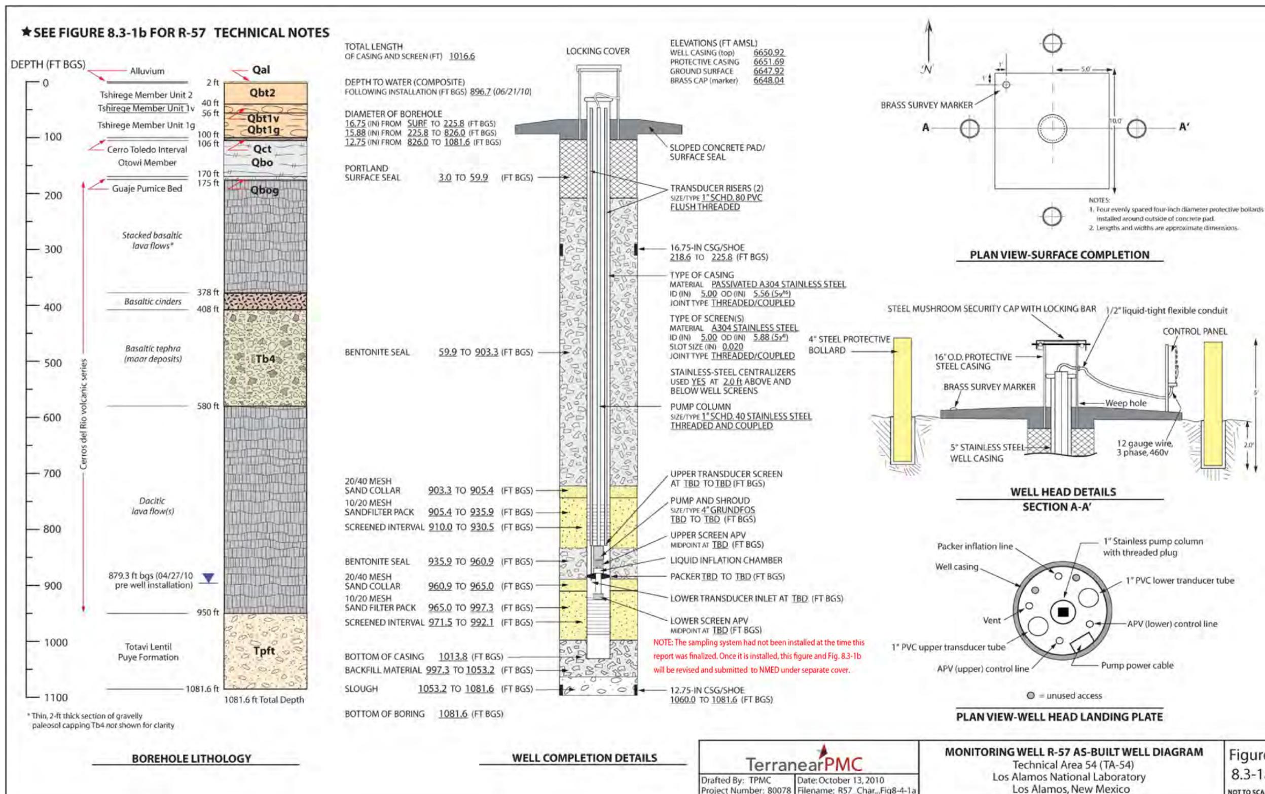
Figure 8.3-1a As-built schematic for regional aquifer monitoring well R-57
