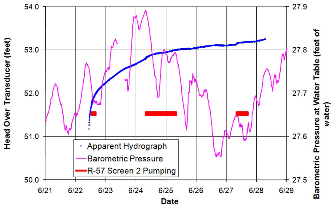
Figure C-7.0-5 Well R-57 screen 1 apparent hydrograph during screen 2 test – full scale
