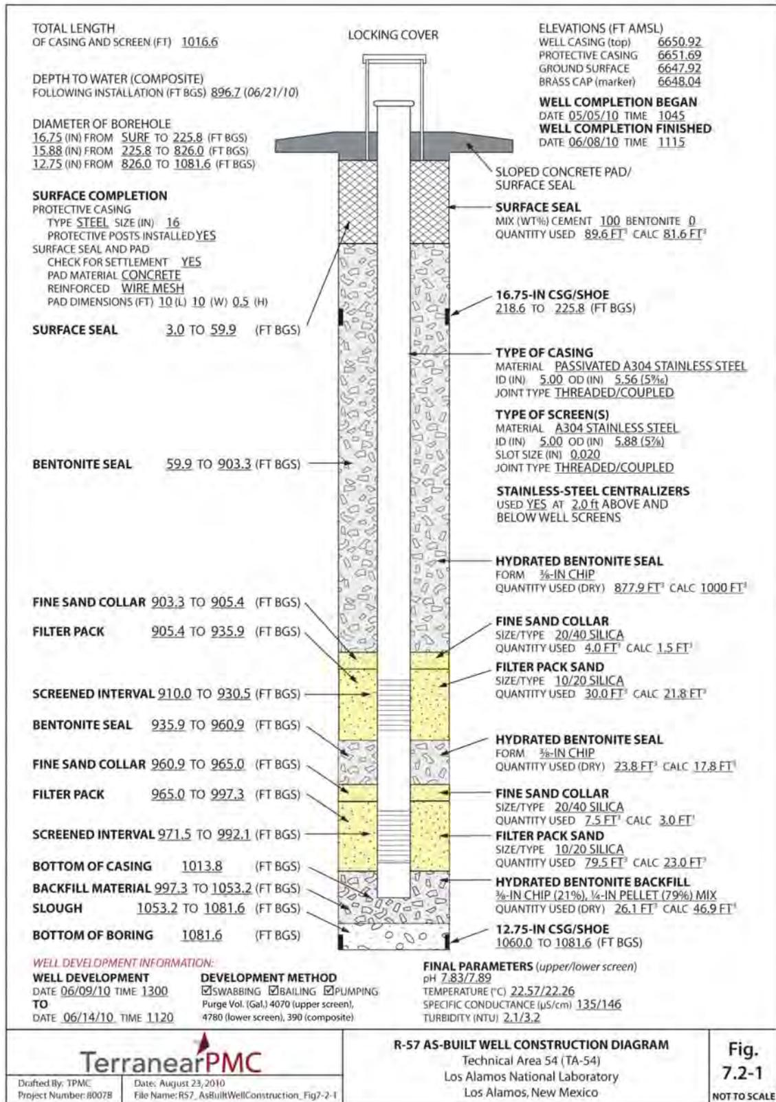
Figure 7.2-1 Monitoring well R-57 as-built well construction diagram
