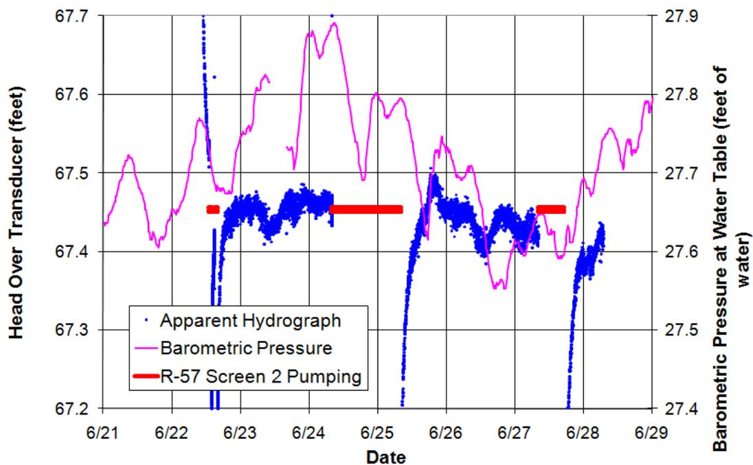
Figure C-7.0-6 Well R-57 screen 2 apparent hydrograph during screen 2 test
