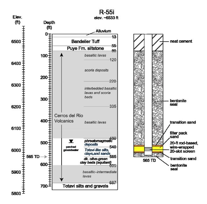
Figure 2 Predicted geology and proposed well design for well R-55i
