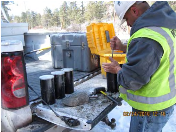
Photo 9 Concrete test cylinders for flume concrete placement
