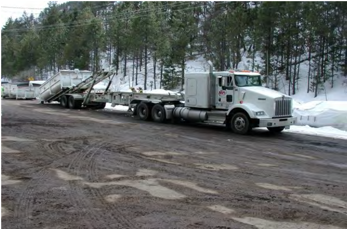
Rolloff bins of excavated rock and sediment being loaded for transport
