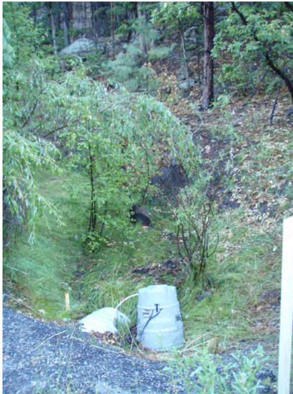
July 2009, Isco sampler at east end of deposition zone before it enters culvert
