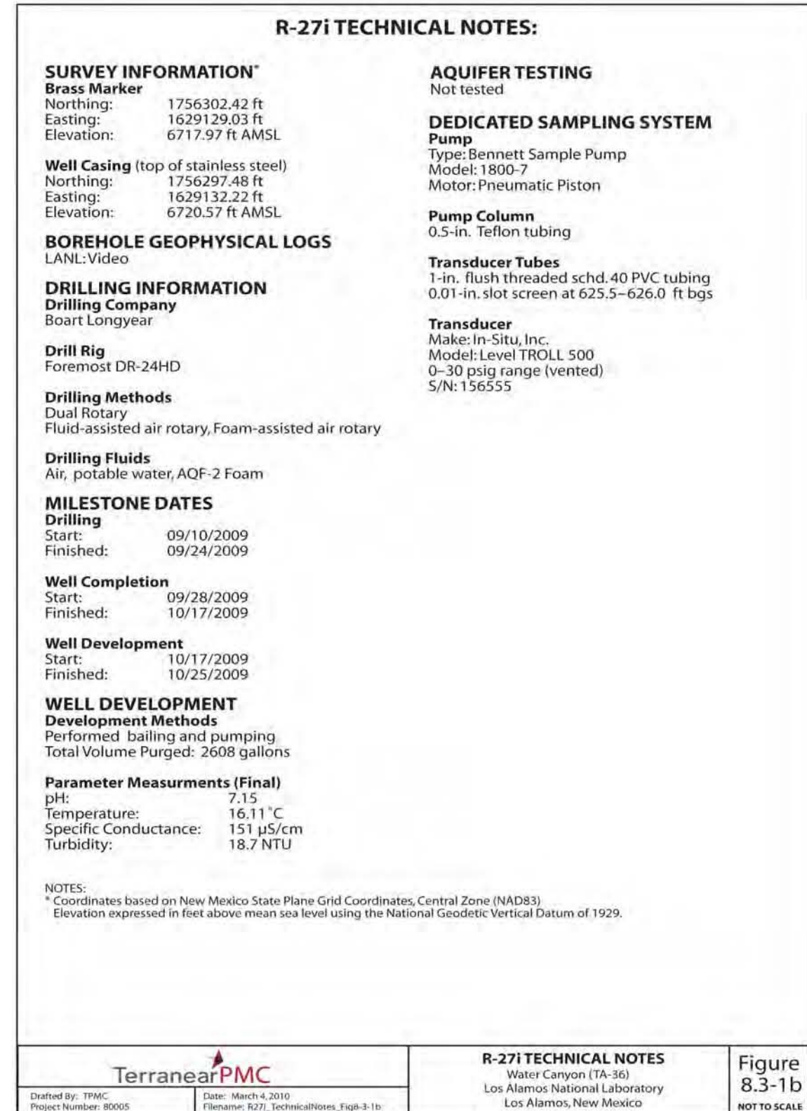
Figure 8.3-1b As-built technical notes for monitoring well R-27
