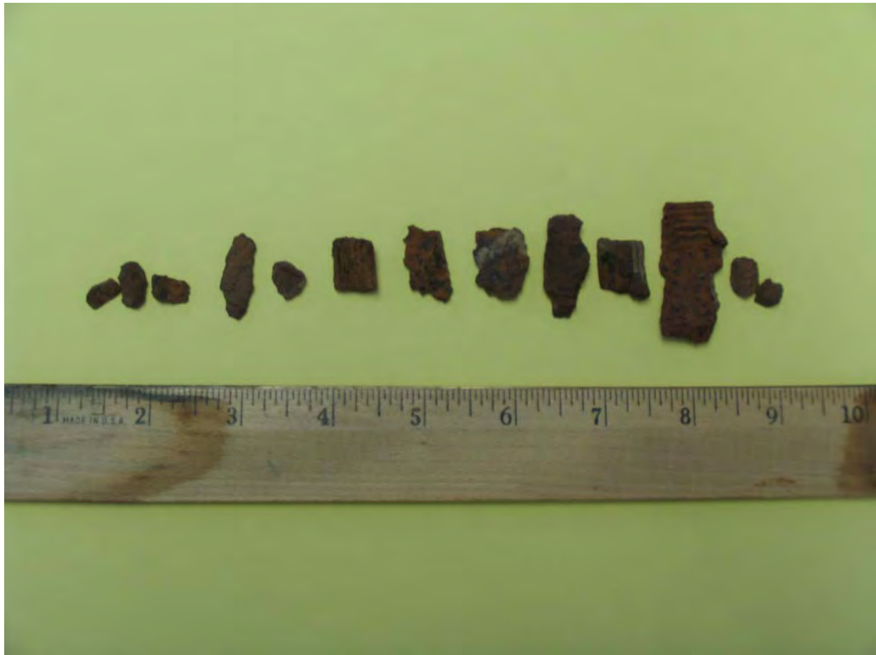
Figure 5.1-3 Miscellaneous small shell fragments found north of the road at SWMU 00-011(a)
