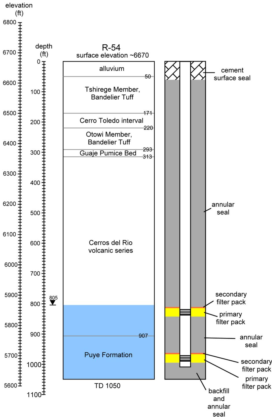
**Figure 2** Predicted geology and well schematic for well R-54
