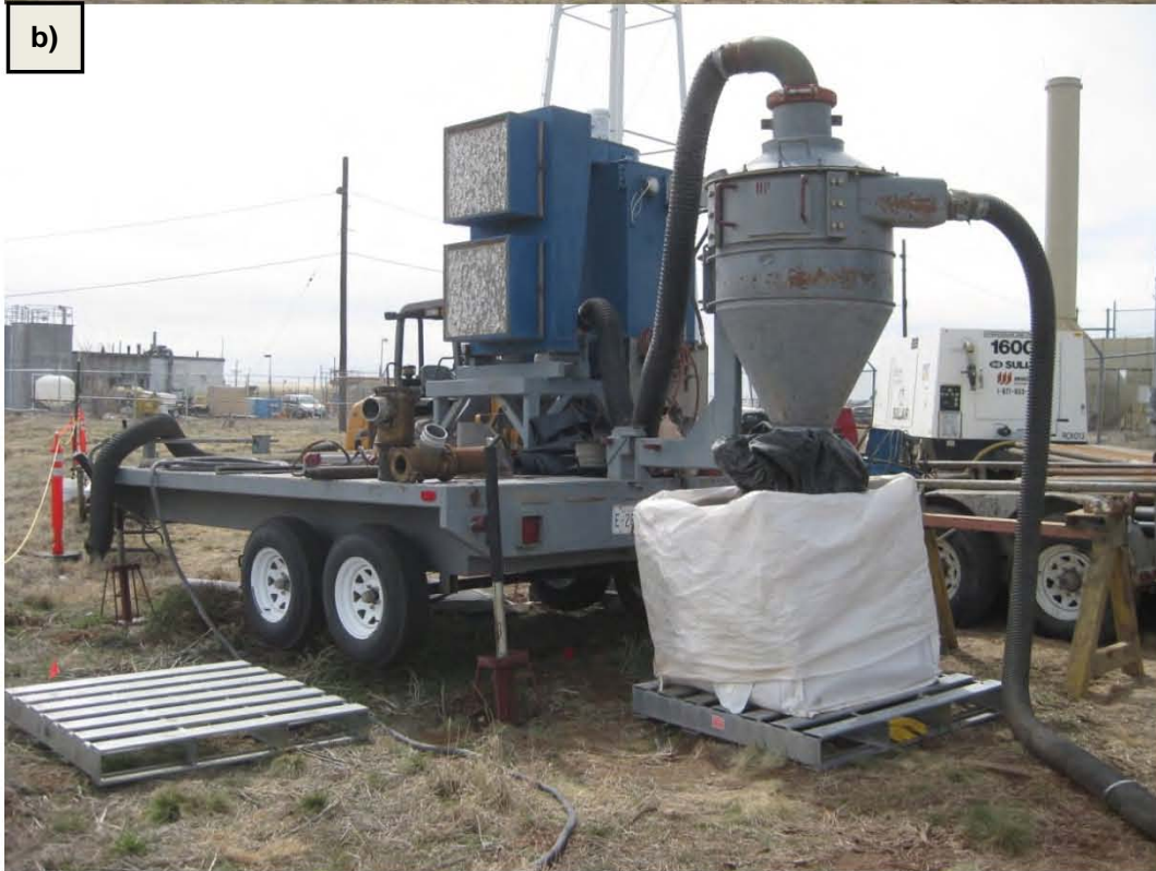
a) General site setup for drilling and sampling at BH 21-25262 b) Dust suppression system utilized during drilling of BH 21-25262
