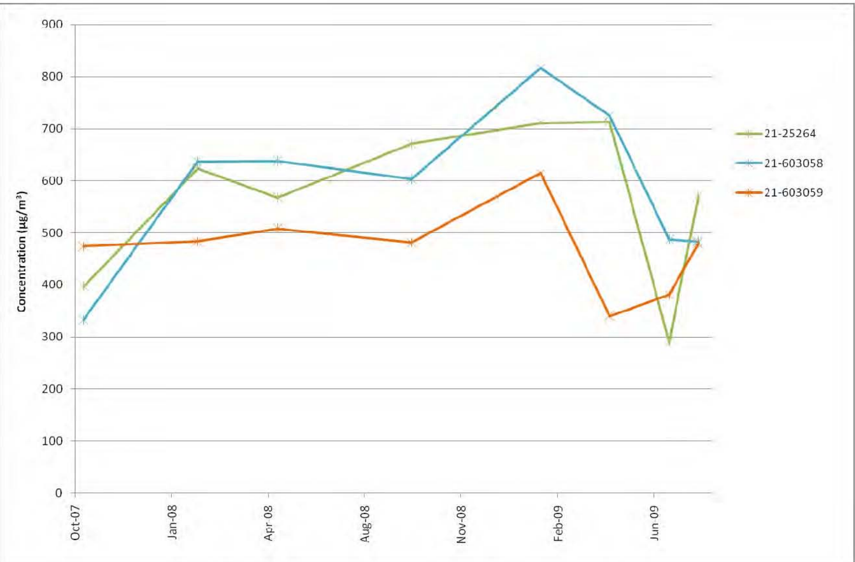
Figure 6.4-6 Time sequence of average VOC concentration (methylene chloride, chloroform, carbon tetrachloride, TCE, and PCE) in vapor-monitoring wells 21-25264, 21-603058, and 21-603059
