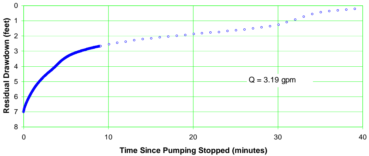
Figure C-9.4-6 Well R-41 screen 2 linear recovery—expanded scale
