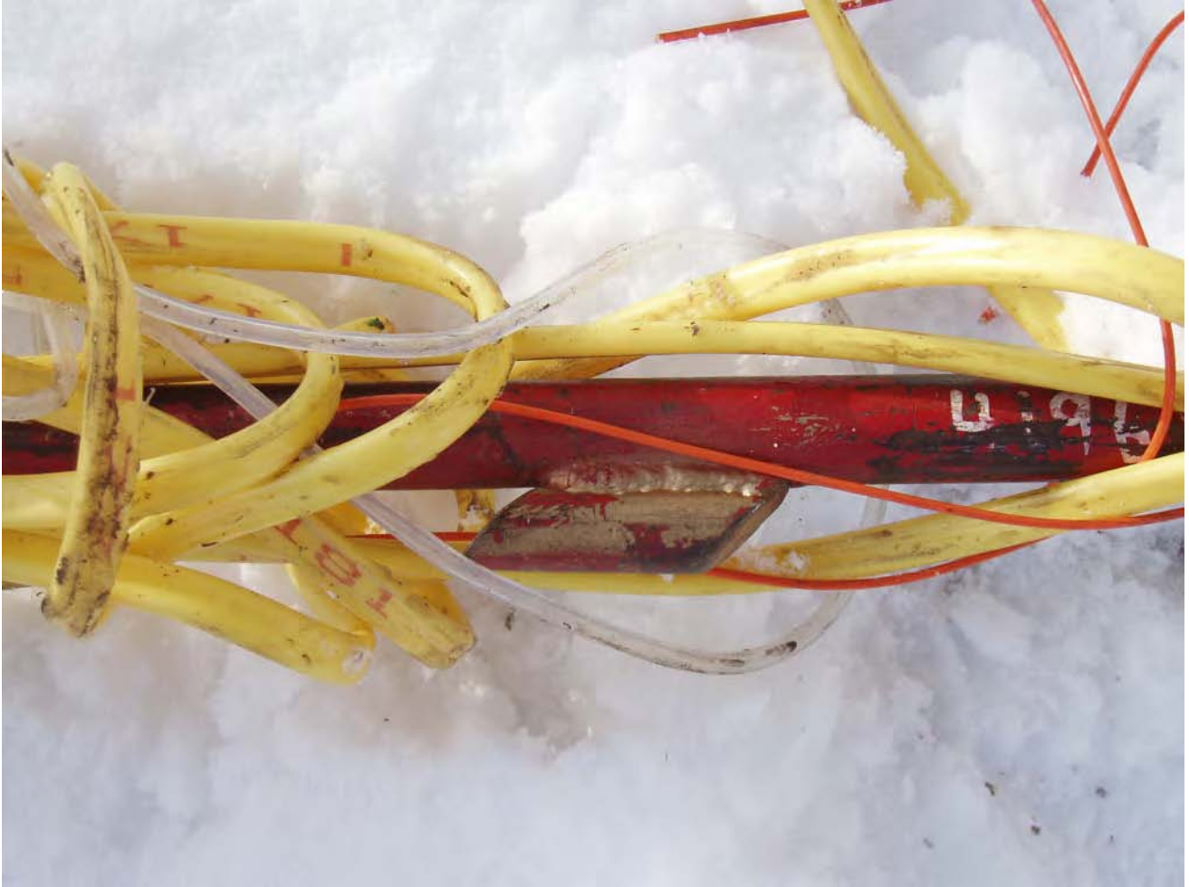
Figure 2.1-4 Fishing tool at R-33 with retrieved Barcad tubing
