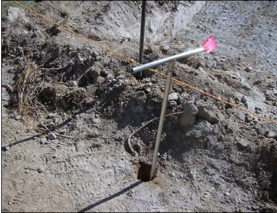
Photo 17 Sampling using hand auger, August–September 2007
