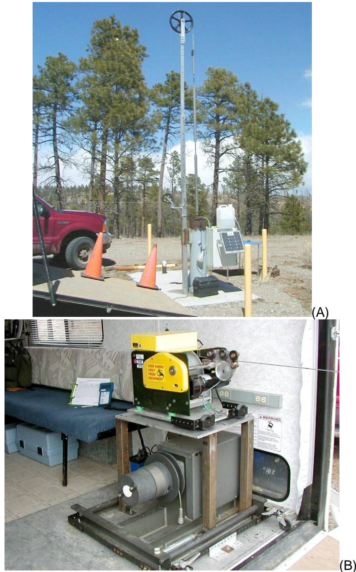
Figure 2-3 (A) Hoist mechanism used for Westbay sampling; (B) Winch mechanism that operates sampling device
