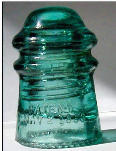
**Fig. 4-2. Hemingray No. 9.** This small blue glass insulator was the type first used on the Jemez Forest Reserve in 1906. Note the drip points around the bottom and the threads that allowed the insulator to be screwed onto the bracket.
