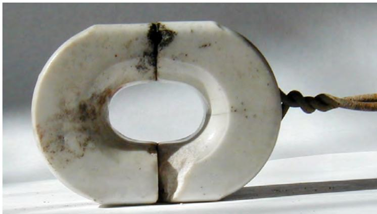
**Fig. 4-11. Thomas Flat-sided Oval. This large white insulator was recognizable because of its flat sides. (GPS waypoint PT68)**
