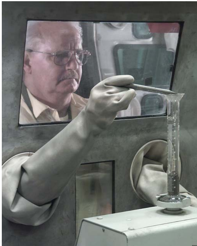
Ed Wilson, NMT-2, does a tap density operation on material bound for Savannah River.
