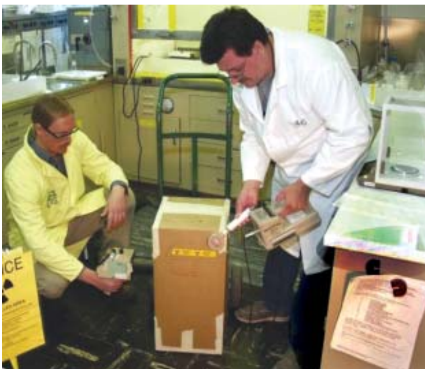
LLW is packaged and surveyed before disposal.
