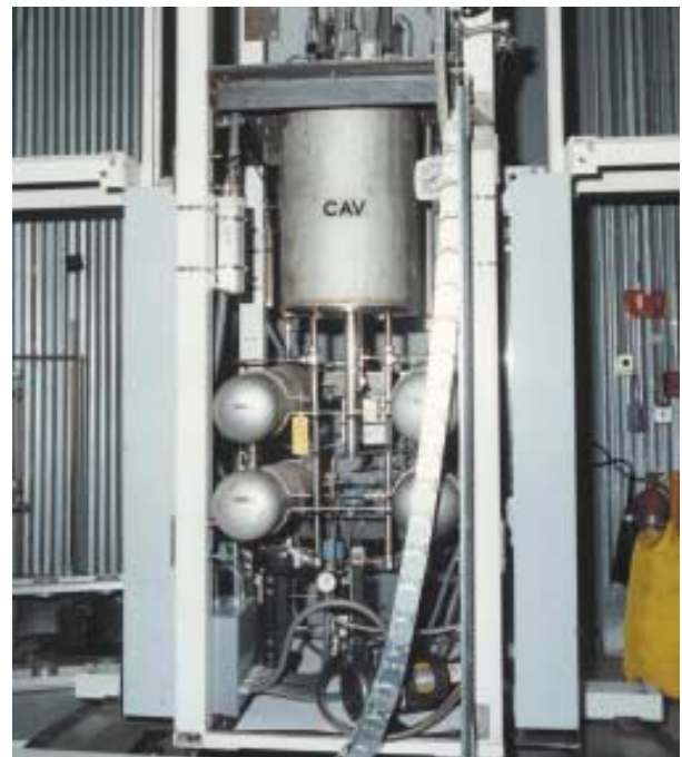
Top: Criticality experiment being setup Bottom: SHEBA is used for criticality testing of nuclear materials in liquid solutions
