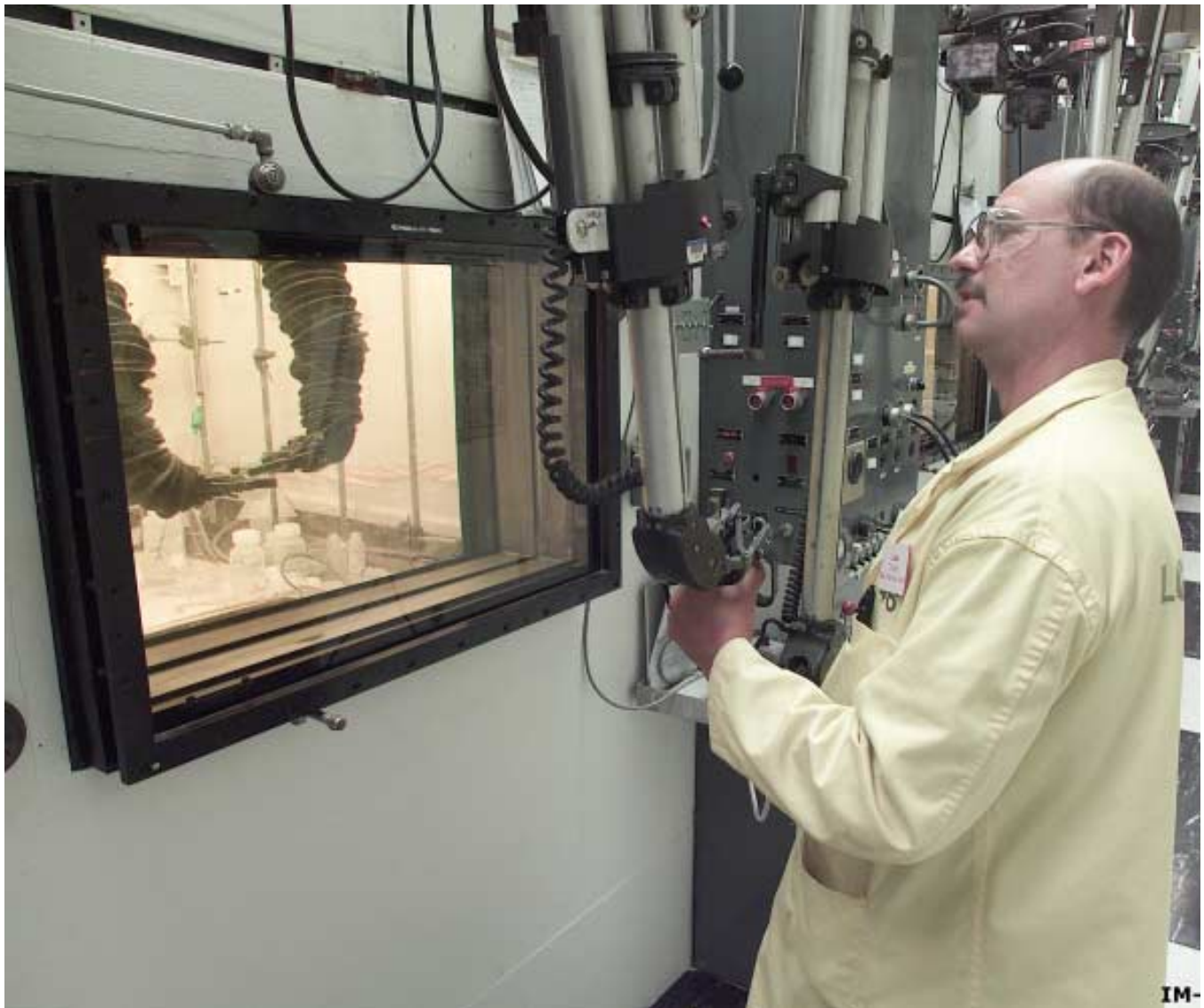
Target material from Russia is handled in a hot cell with mechanical manipulators
