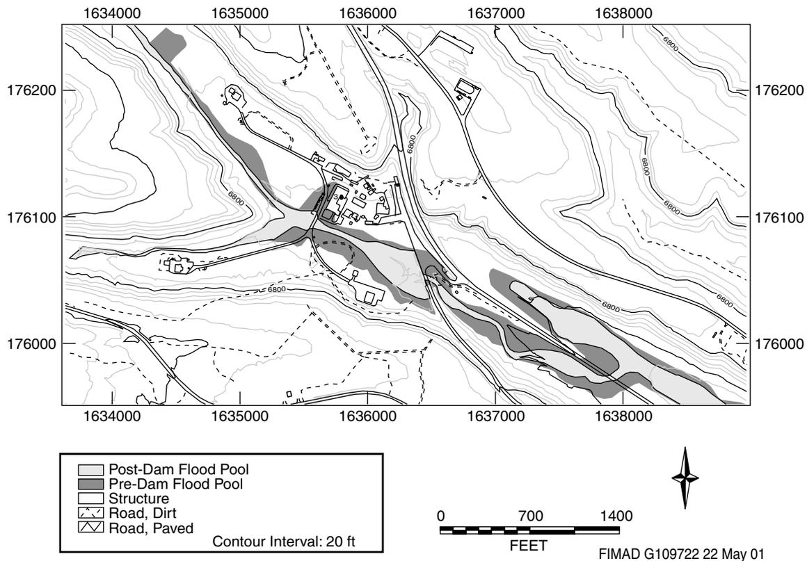
Figure 10. Predicted post-fire 100 year floodpool map at Technical Area 18 before and following construction of the upstream Pajarito flood control structure
