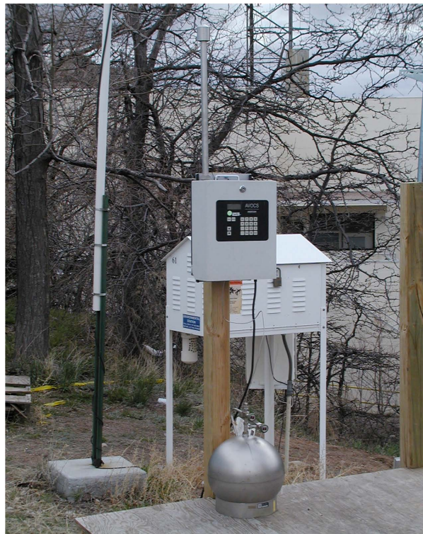
Figure 4-2. Ambient Volatile Organic Collection System at Site #61.
