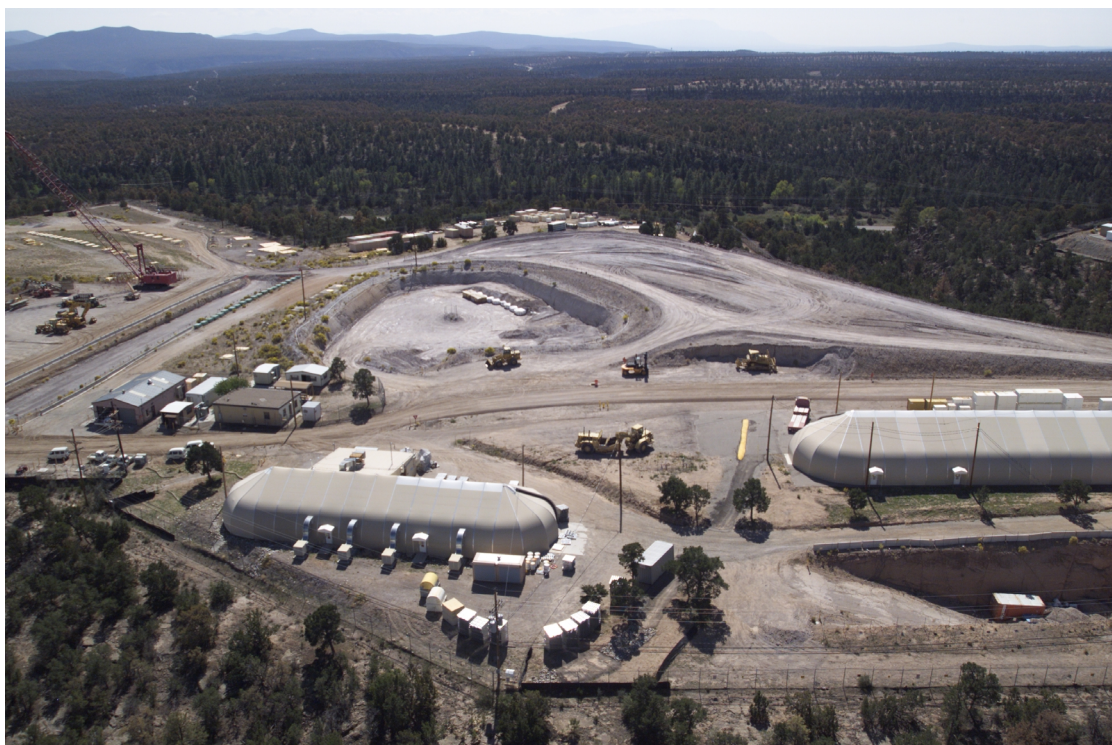
Figure 4. Aerial photo of Area G showing the membrane-covered domes used to handle waste. Also visible are pits and trenches containing low-level radioactive waste packages.
