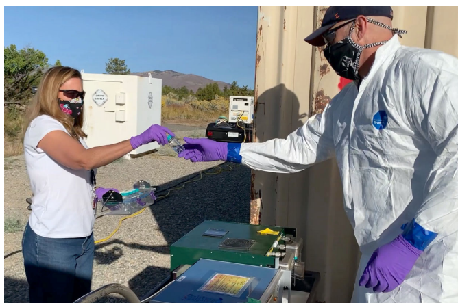
Laboratory engineers have done a careful analysis of the venting process to ensure that any releases are carefully controlled. The system pictured here, has been specifically engineered to capture the form of tritium expected in the FTWC headspace.
