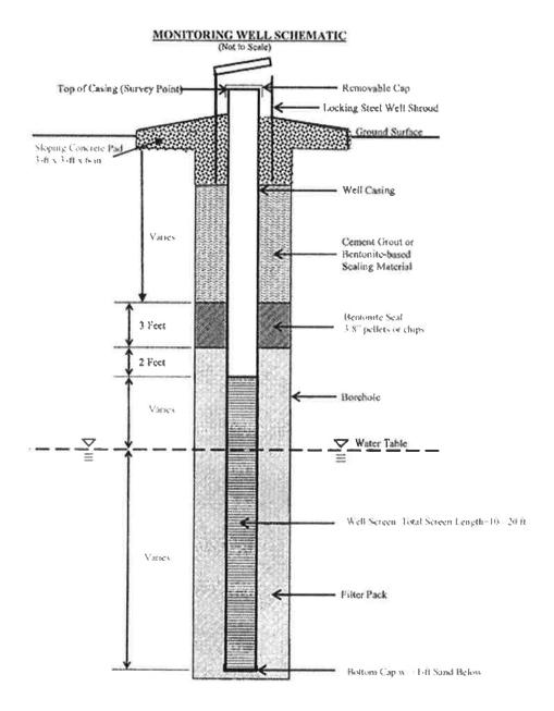
Figure 2.0. Conceptual Design, Alluvial Monitoring Well
