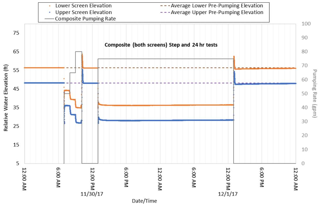
**Figure D-1.0-2** Relative water elevation above transducers (left axis) and pumping rate (right axis) throughout the duration of the CrEX-4 composite pumping tests
