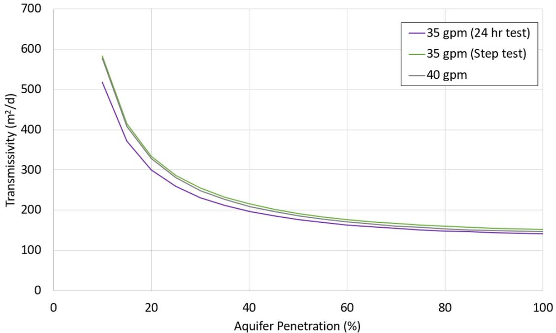
Figure D-3.0-8 Transmissivities calculated using the MATLAB code of McLin (2005, 602537), based on the specific capacity method, for each step of the upper-screen variable-rate pumping test (35 and 40 gpm) and the 24-h test (35 gpm) as a function of aquifer penetration
