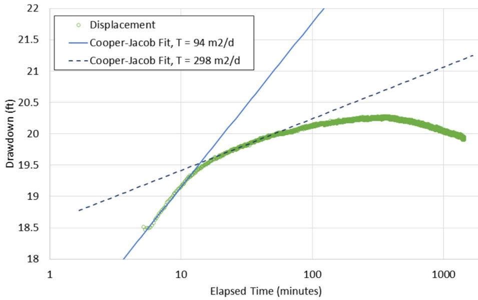
**Figure D-3.0-3** Corrected drawdown data (spikes removed) and multiple fits from AQTESOLV for the Cooper-Jacob solution to the composite 24-h pumping test
