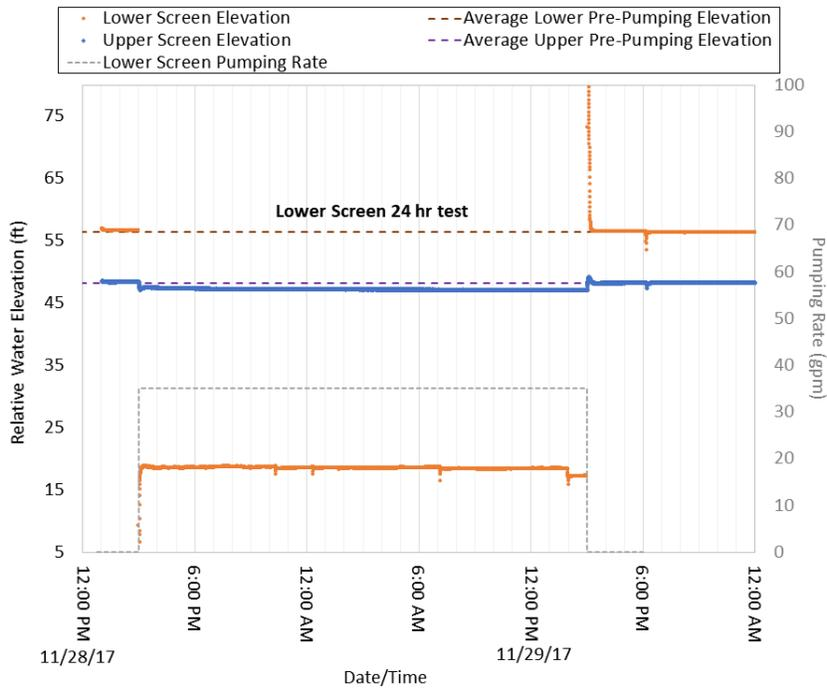
**Figure D-1.0-1** Relative water elevation above transducers (left axis) and pumping rate (right axis) throughout the duration of the CrEX-4 lower-screen 24-h pumping test
