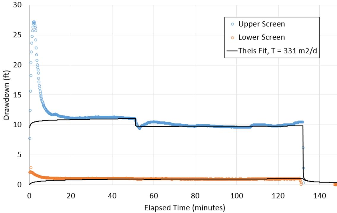
Figure D-3.0-7 Drawdown data and the best fit from AQTESOLV for the Theis solution to the upper-screen step test,  $T = 331 \text{ m}^2/\text{d}$
