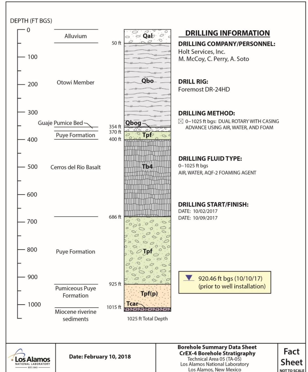
Figure 5.1-1 Extraction well CrEX-4 borehole stratigraphy
