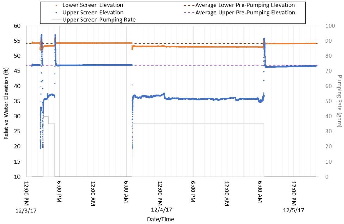
**Figure D-1.0-3** Relative water elevation above transducer (left axis) and pumping rate (right axis) throughout the duration of the CrEX-4 upper-screen pumping tests
