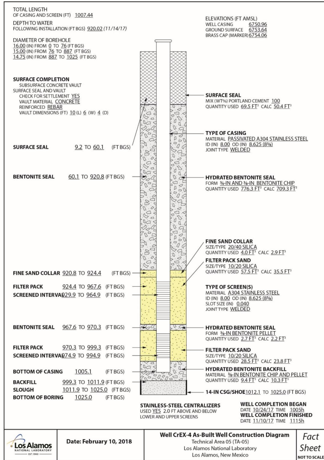
Figure 7.2-1 Extraction well CrEX-4 as-built well construction diagram
