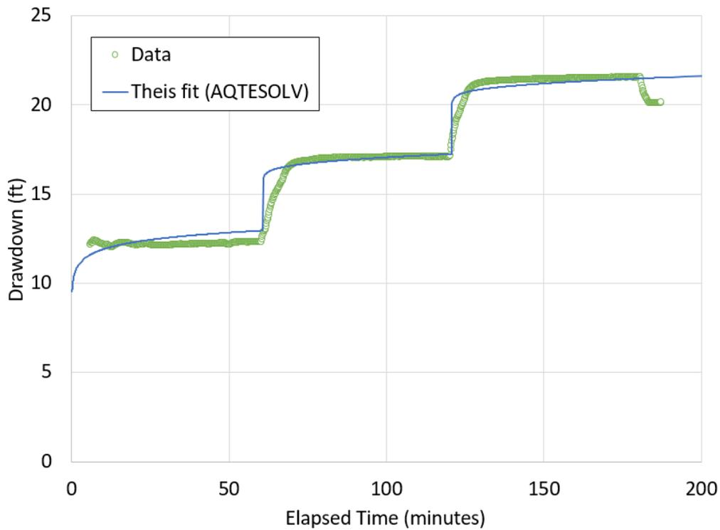
**Figure D-3.0-4** Drawdown data (spikes removed) and the best fit from AQTESOLV for the Theis solution to the composite step test,  $T = 122 \text{ m}^2/\text{d}$
