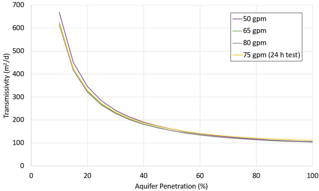
**Figure D-3.0-5** Transmissivities calculated using the MATLAB code of McLin (2005, 602537), based on the specific capacity method, for each step of the composite variable-rate pumping test (50, 65, and 80 gpm) and the 24-h test (75 gpm) as a function of aquifer penetration
