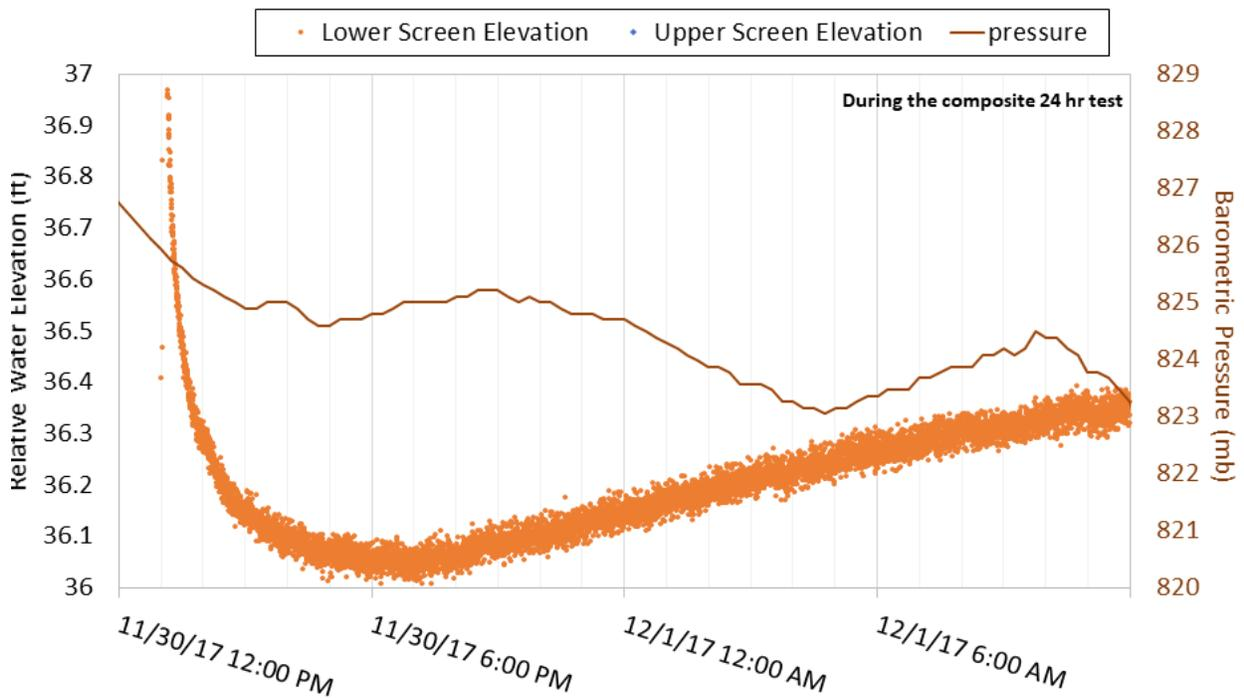
**Figure D-1.0-4** Relative water elevation above transducer (left axis) and barometric pressure (right axis) during the CrEX-4 lower-screen and composite pumping tests
