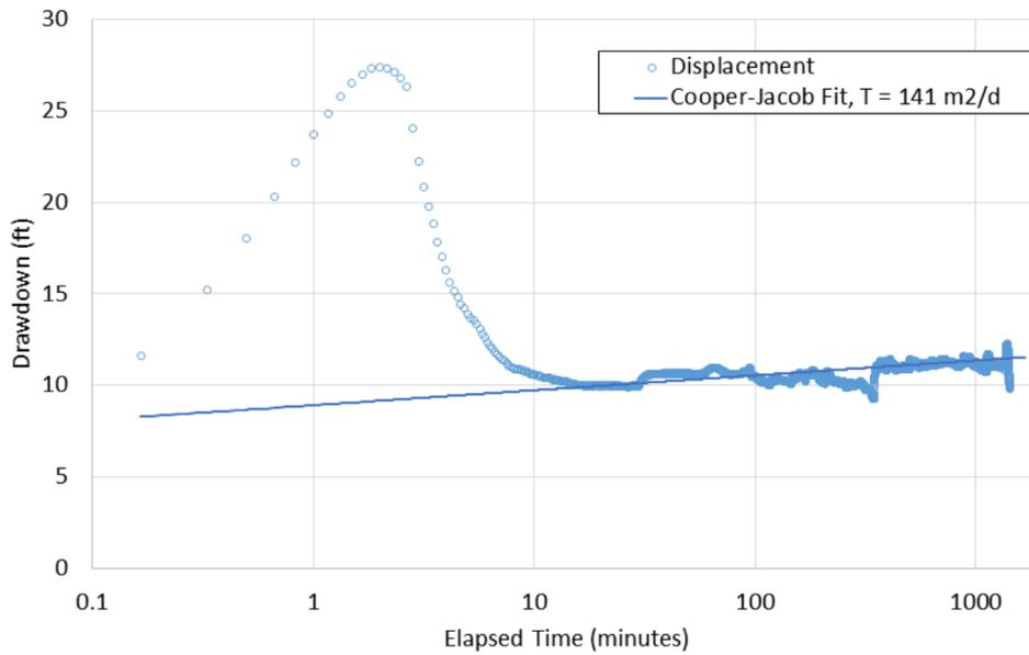
**Figure D-3.0-6** Complete drawdown data (spike not removed) and fit from AQTESOLV for the Cooper-Jacob solution to the upper-screen 24-h pumping test
