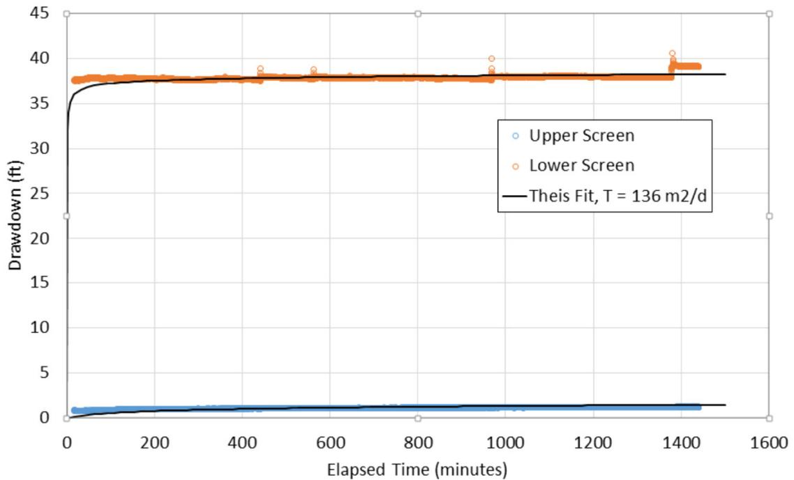
**Figure D-3.0-2** Corrected drawdown data for both screens (spikes removed) and the Theis fit from AQTESOLV for the lower-screen 24-h pumping test,  $T = 136 \text{ m}^2/\text{d}$
