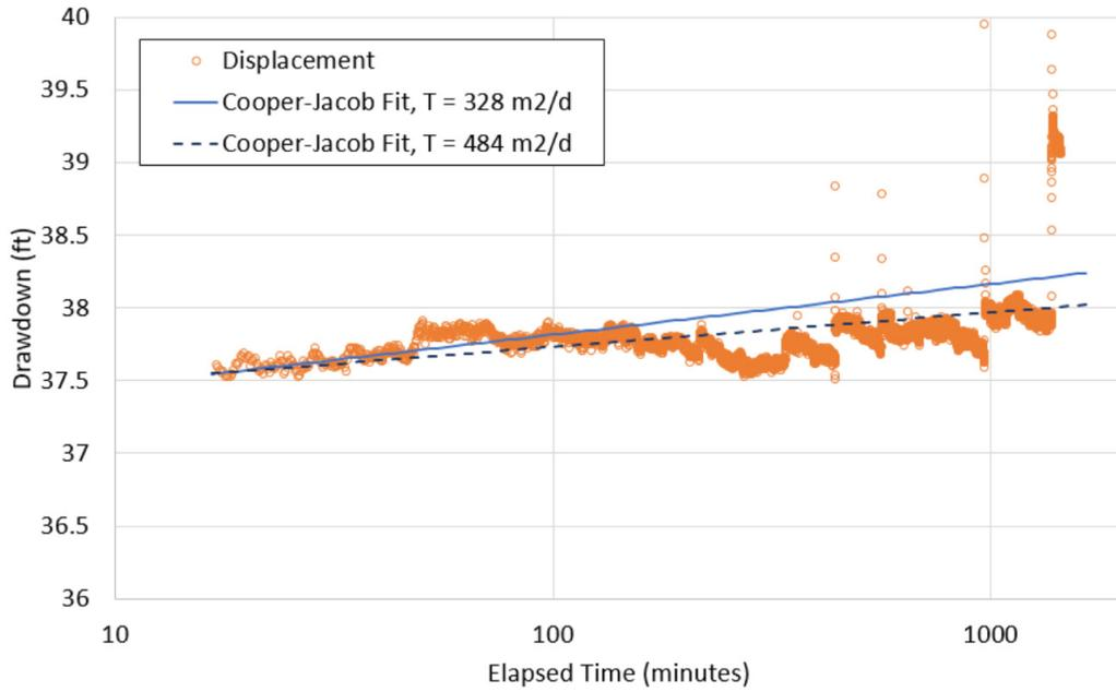
**Figure D-3.0-1** Corrected drawdown data (spikes removed) and multiple fits from AQTESOLV for the Cooper-Jacob solution to the lower-screen 24-h pumping test
