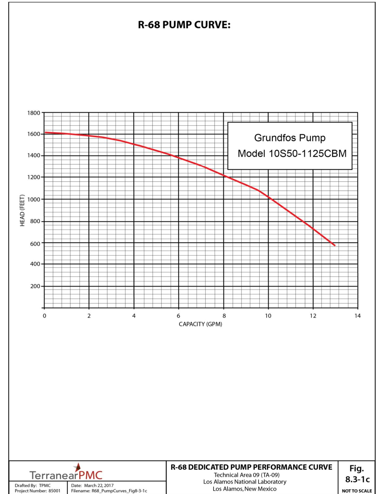
Figure 8.3-1c Pump curve for monitoring well R-68
