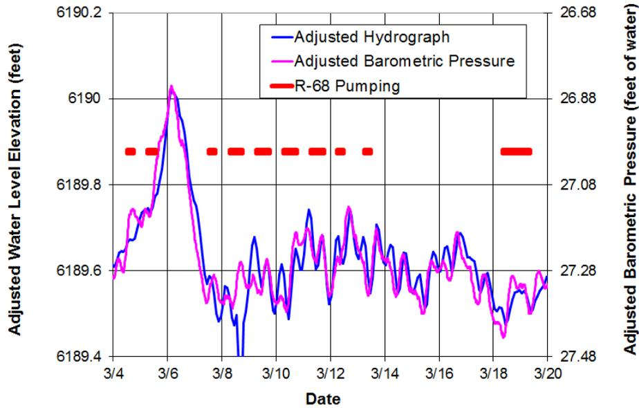
Figure E-7.0-3 Well R-63 adjusted hydrograph for 88% barometric efficiency and 0.002 ft/d water level rise
