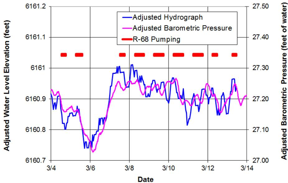
Figure E-7.0-6 Well R-25 screen 7 adjusted hydrograph for 60% barometric efficiency and 0.013 ft/d water level decline
