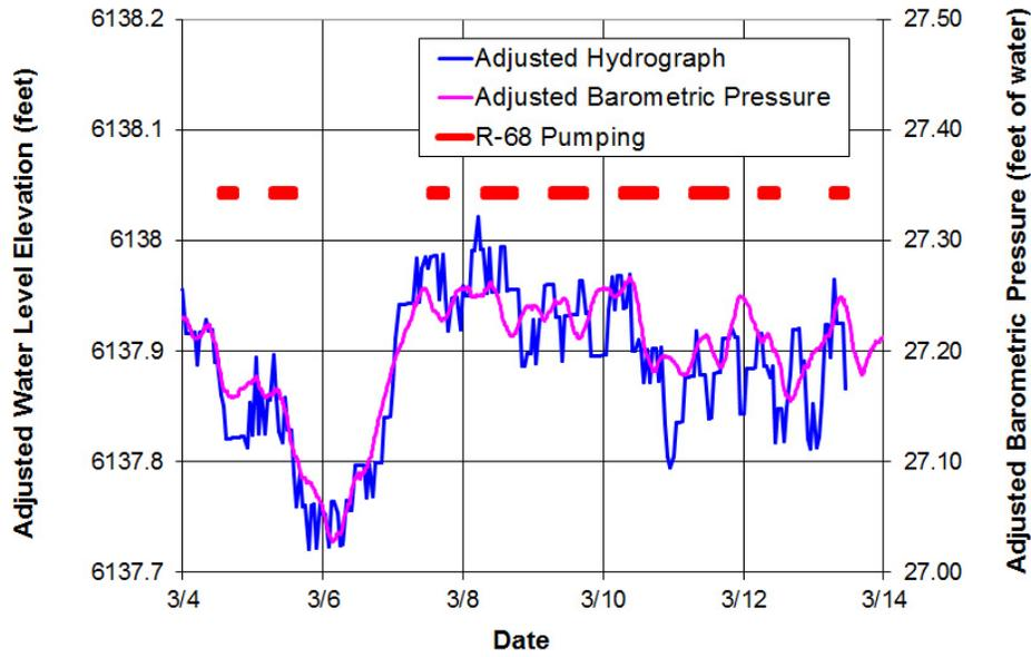
Figure E-7.0-7 Well R-25 screen 8 adjusted hydrograph for 60% barometric efficiency and 0.013 ft/d water level decline
