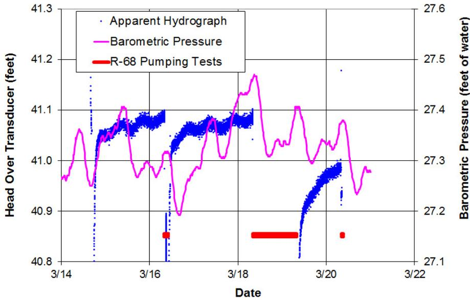
Figure E-7.0-1 Well R-68 apparent hydrograph and barometric pressure
