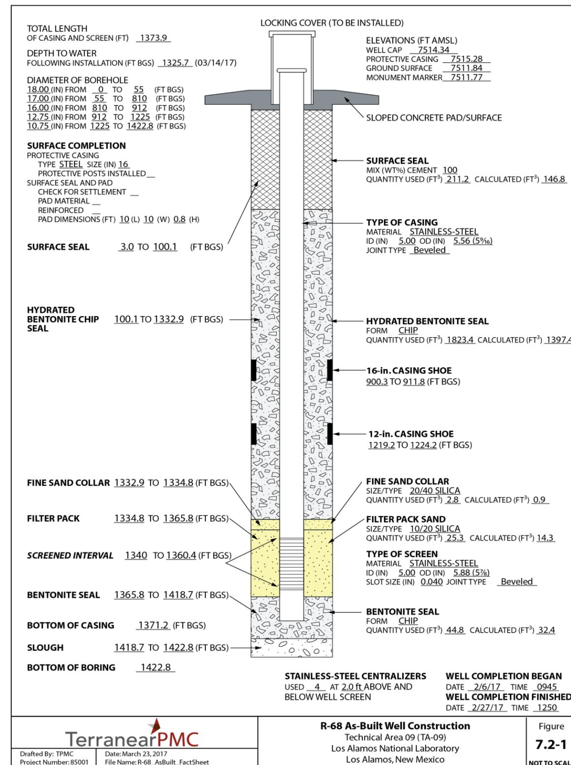
Figure 7.2-1 Monitoring well R-68 as-built well construction diagram
