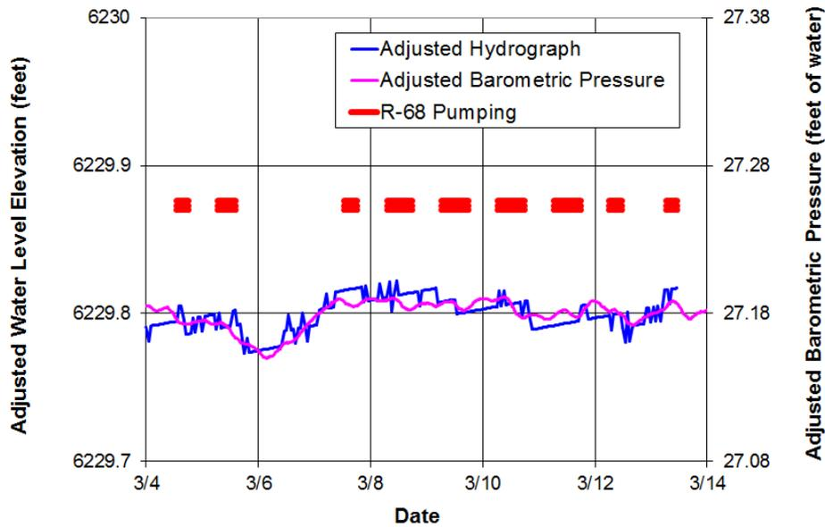
Figure E-7.0-4 Well R-25 screen 5 adjusted hydrograph for 93% barometric efficiency and 0.007 ft/d water level decline
