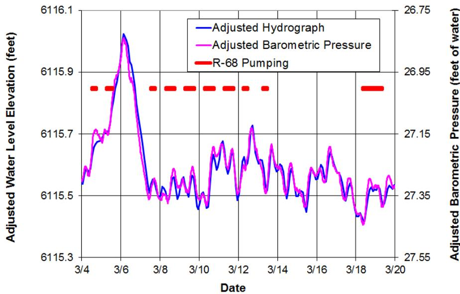
Figure E-7.0-2 Well R-18 adjusted hydrograph for 91% barometric efficiency and 0.003 ft/d water level decline
