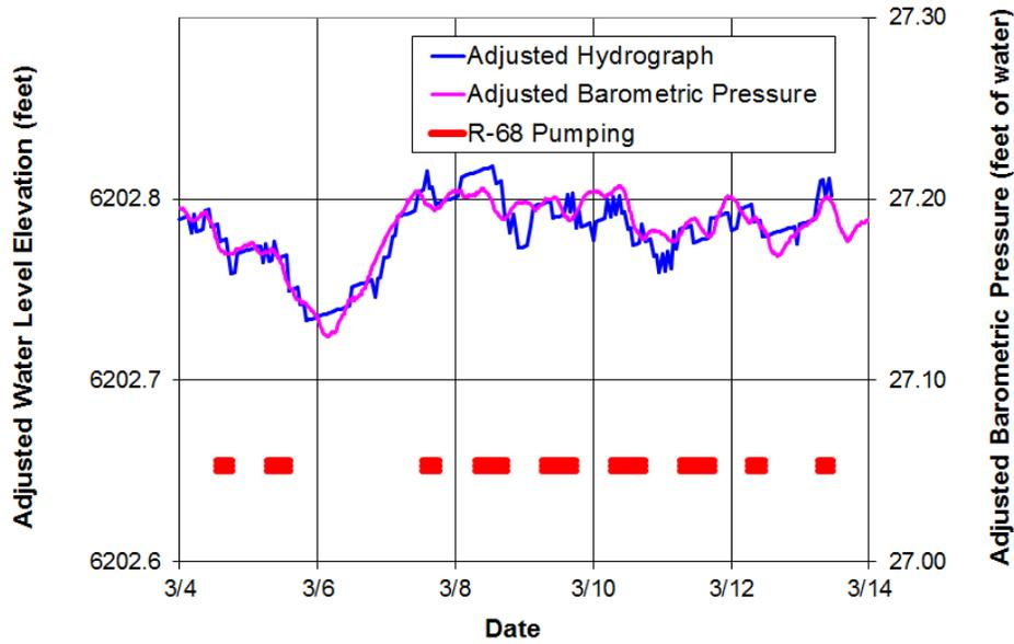
Figure E-7.0-5 Well R-25 screen 6 adjusted hydrograph for 86% barometric efficiency and 0.013 ft/d water level decline
