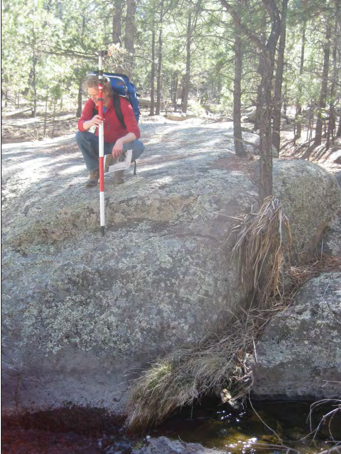
Photo B1-5 Location of maximum elevation change (+5.5 ft) detected. No actual geomorphic change occurred. This boulder at the eastern end of reach S-2 was classified as ground in 2016 but not in 2015. March 2017 photo looking south.
