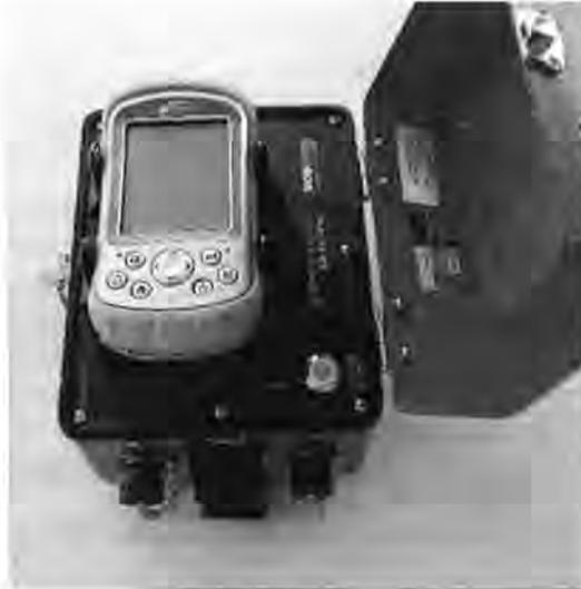
Figure 3-1 GK405 Readout Unit
