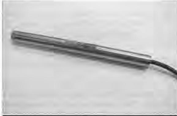
The Model 4500 AR piezometer is designed to be used with readouts systems that can read frequency but do not have the capability to "pluck" the VW gage. This sensor has built-in electronics that cause the gage wire to vibrate in a continuous mode at its resonant frequency. The output from the sensor is a 5 volt DC square wave at this frequency.
