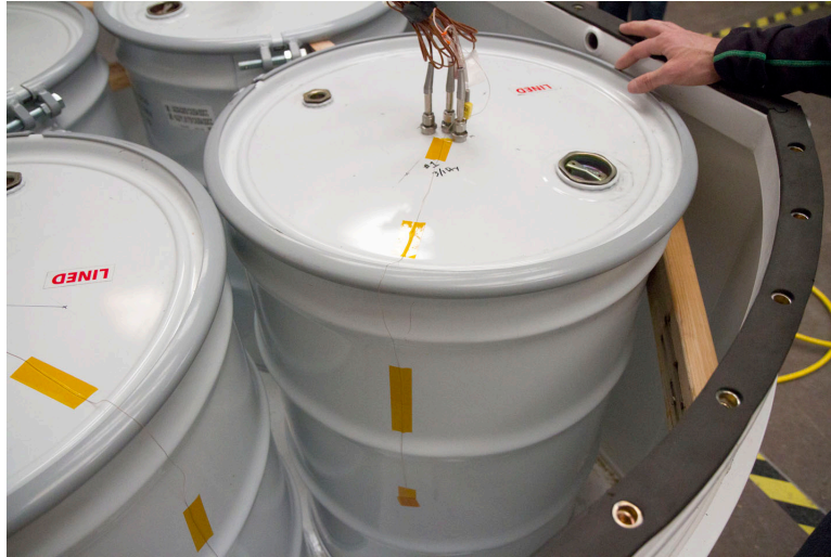
Figure 3. A closed drum with 3 thermocouple probes inserted through the lid and 1 thermocouple attached with orange tape on the external surface.
