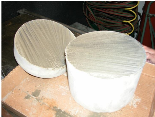
Figure 8 Cut specimen of cemented surrogate nitrate salt/Swheat
