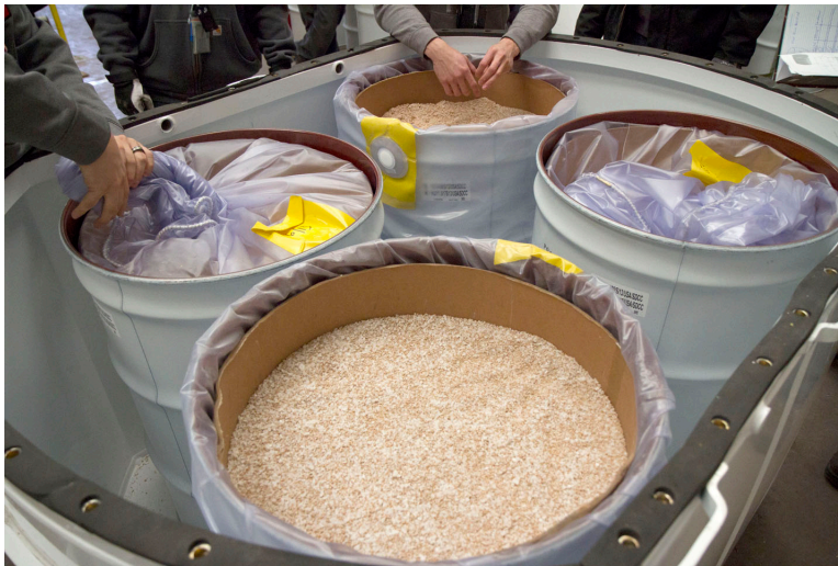
Figure 2. The four drums, nested in the SWB and filled with the kitty litter and rock salt mixture. The plastic bag and cardboard liner system is visible.
