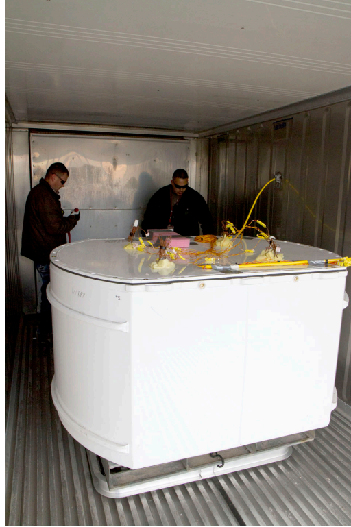
Figure 6. The SWB placed within the freezer unit. Thermocouple extension cables have been connected.
