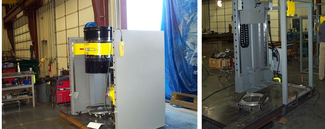
Figure 25 Daughter drum and waste drum lifts for MORK
