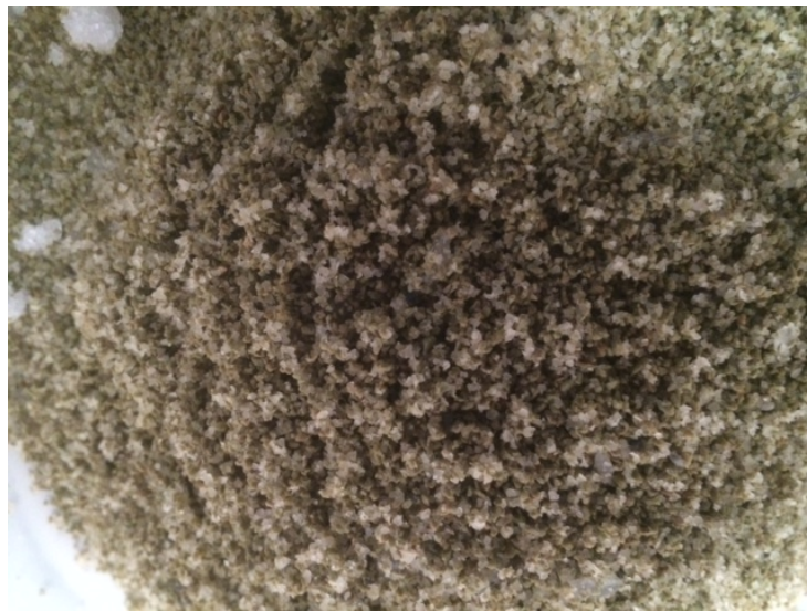
Figure 8 Waste Lock 770 surrogate waste blended with zeolite (Test WL 13)
