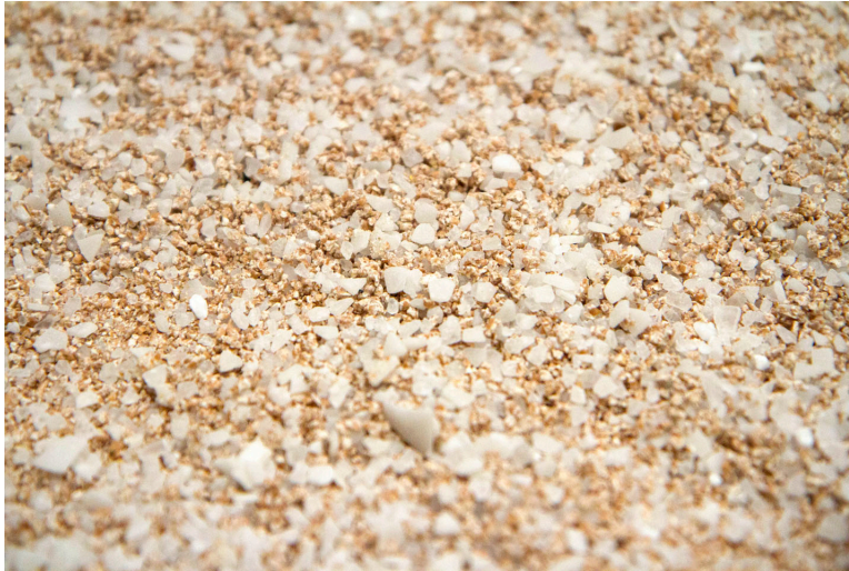
Figure 1. A mixture of Swheat™ kitty litter and SafeStep™ Enviro-Blend Power 6300 rock salt used in this study.
