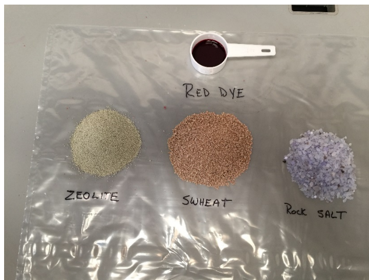
Figure 1. Samples of zeolite, Swheat, rock salt, and dye used for tests
