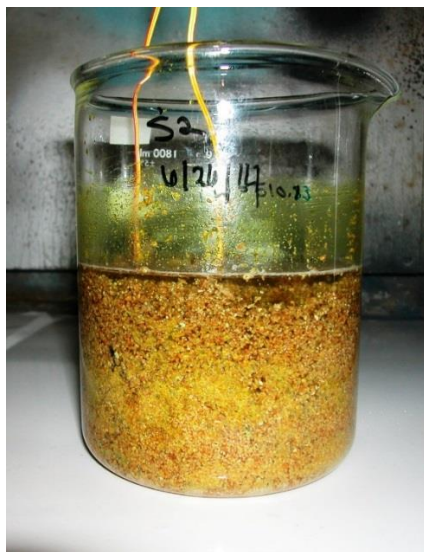
Figure 7 Mixture of nitrate salt, Swheat, and water before cementation
