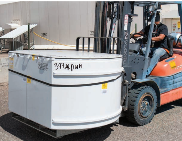
Standard waste boxes contain drums awaiting shipment to WIPP.
