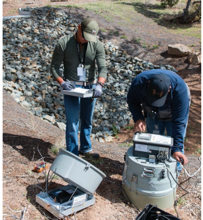
Workers program automated storm-water samplers.
