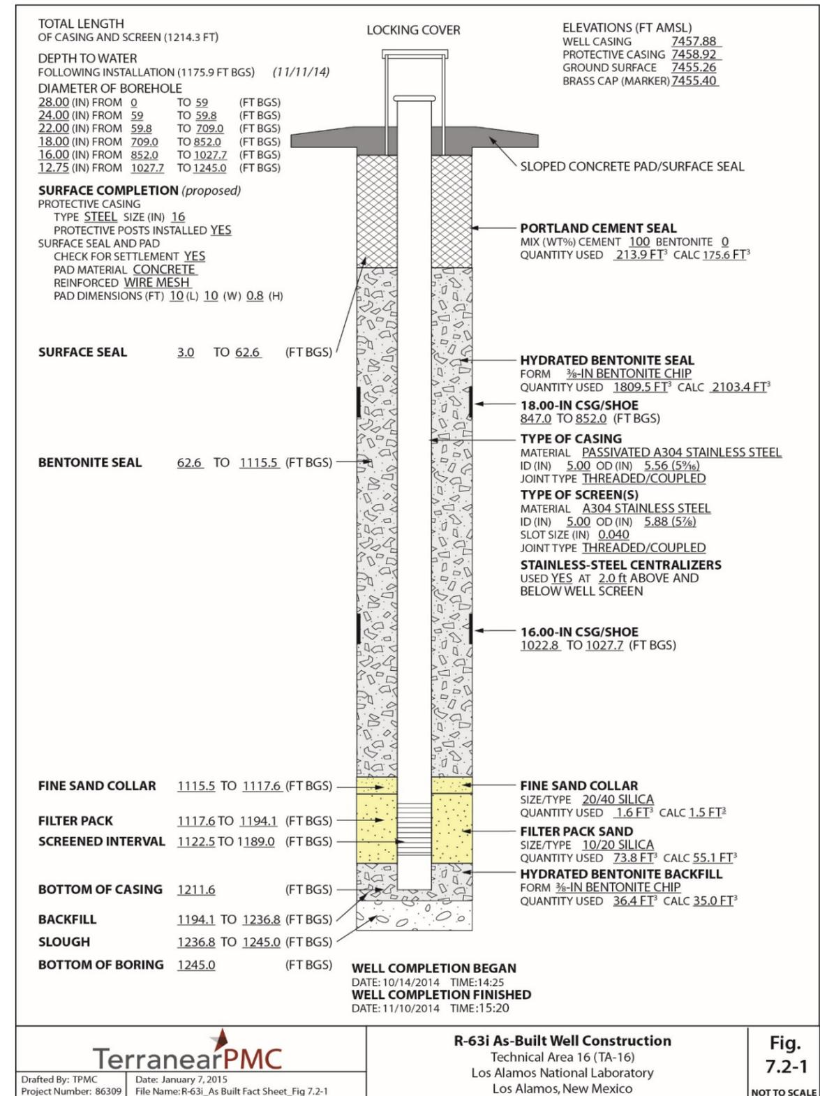
Figure 7.2-1 Monitoring well R-63i as-built well construction diagram
