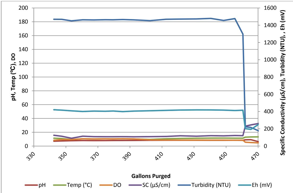
Figure B-2.3-1 Field parameters versus volume purged during R-63i well development
