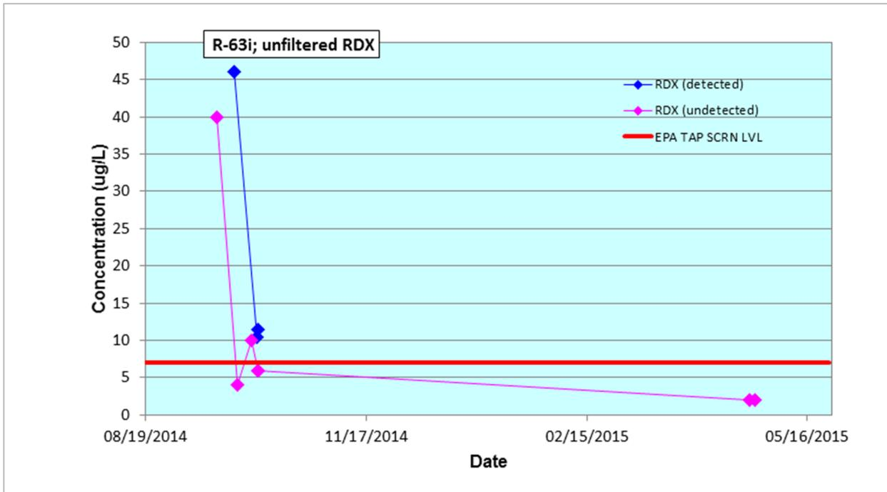
Figure B-2.2-1 RDX sample measurements during R-63i drilling and well development
