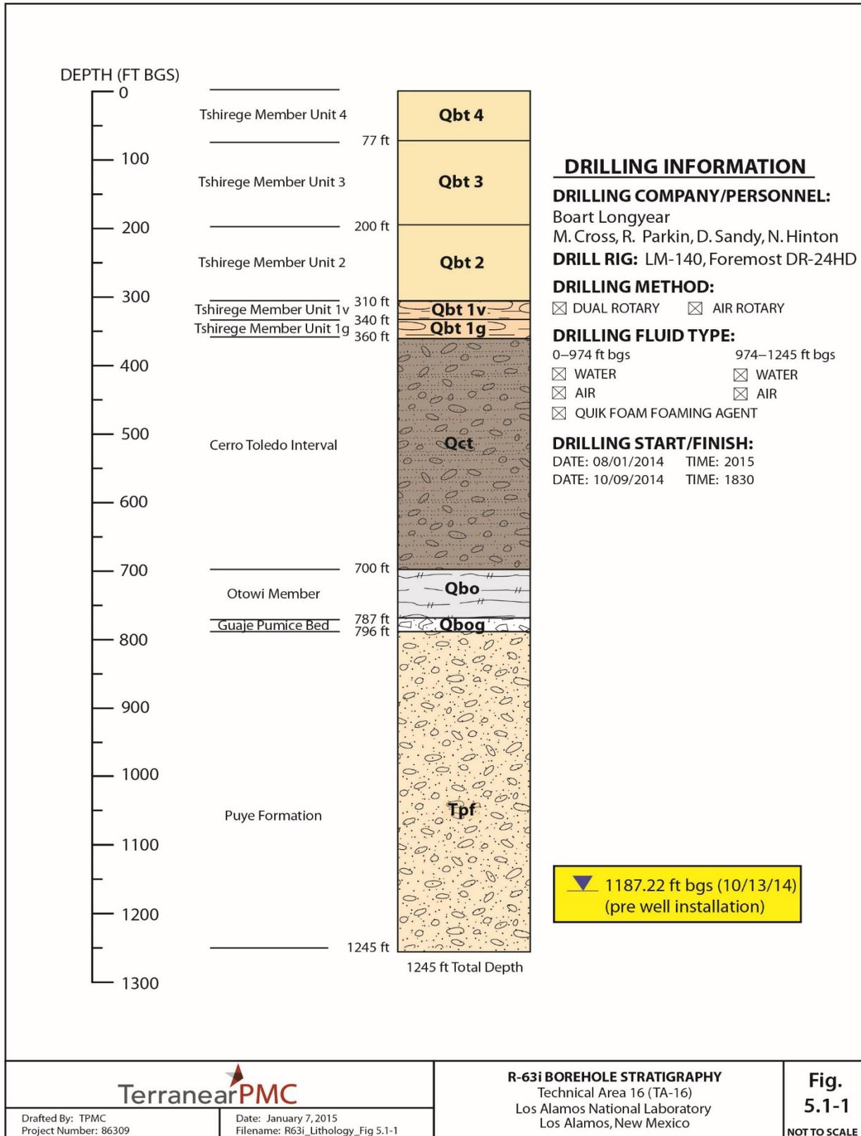
Figure 5.1-1 Monitoring well R-63i borehole stratigraphy
