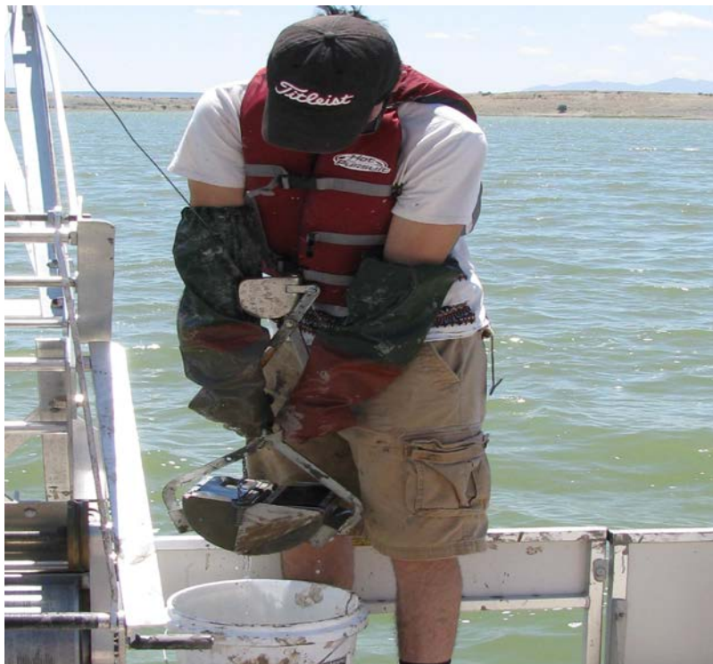
Figure 7-38 Collecting a sediment sample with a Ponar grab sampler
