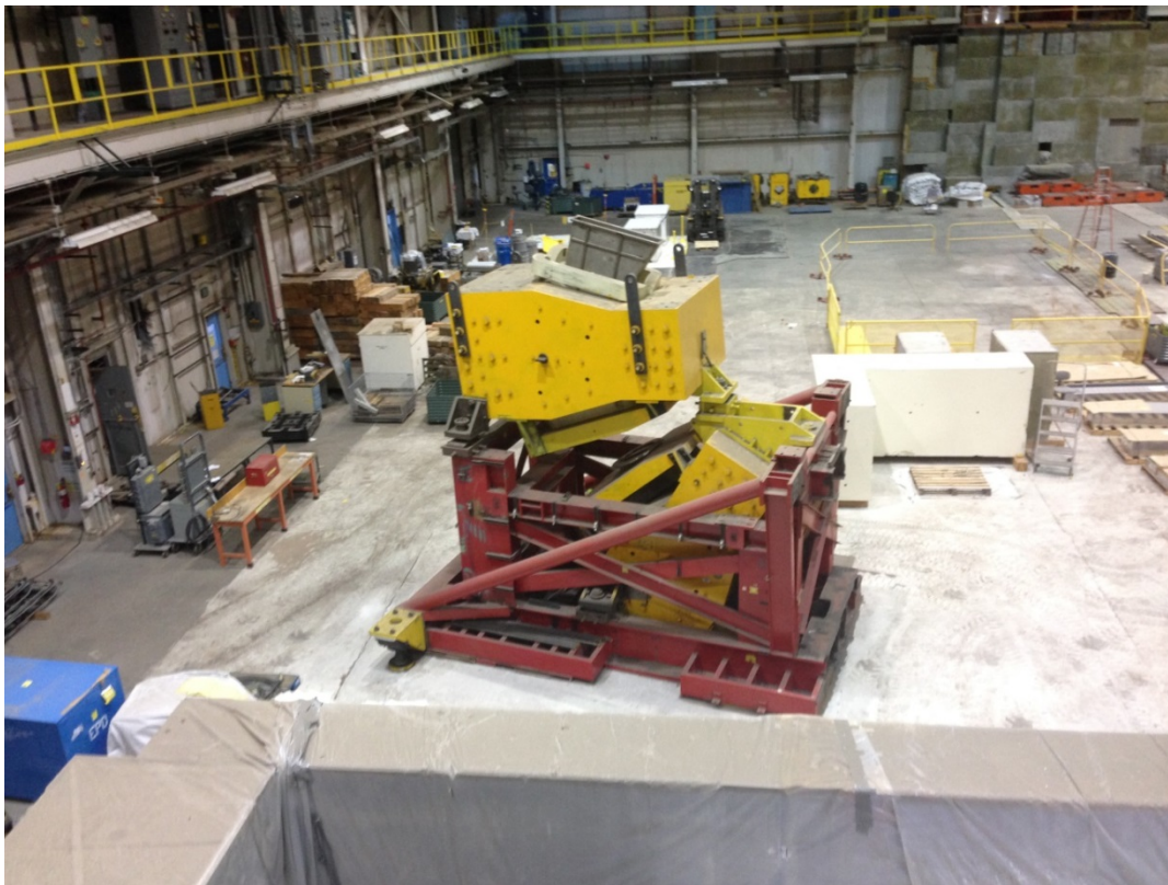
Figure 1-6 EPICS Spectrometer in Area A – over 200 tons of magnet and cold-rolled steel encumbering projected new mission workspace
