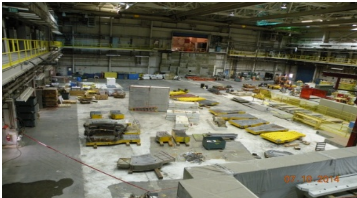
Figure 1-7 Large EPICS spectrometer magnets after initial dismantlement. Each magnet consisted of ten magnet plates, each plate weighing over 10 tons. The Area A space has been repurposed for new experimental activities.
