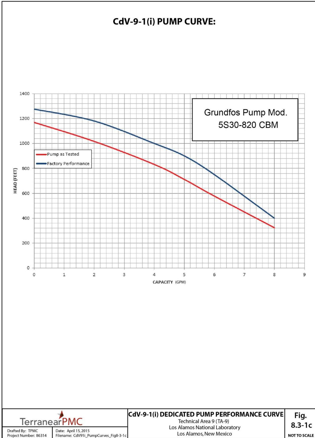
Figure 8.3-1c Pump curves for monitoring well CdV-9-1(i)
