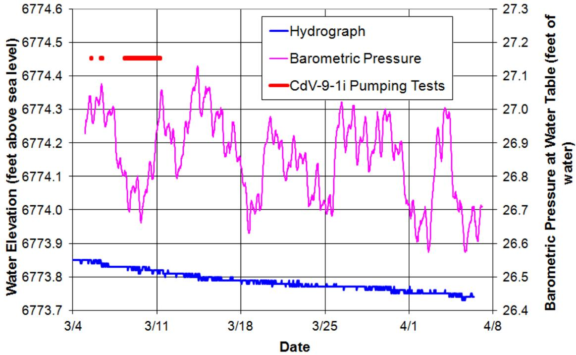
Figure F-8.0-13 Well R-25 screen 1 apparent hydrograph
