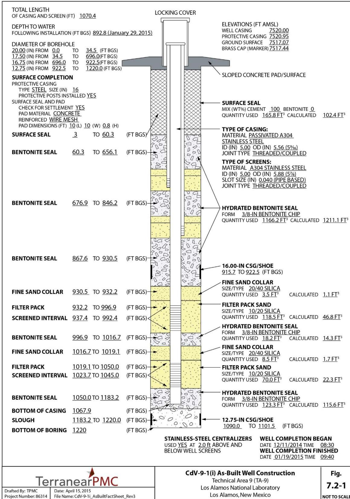
Figure 7.2-1 Monitoring well CdV-9-1(i) as-built well construction diagram
