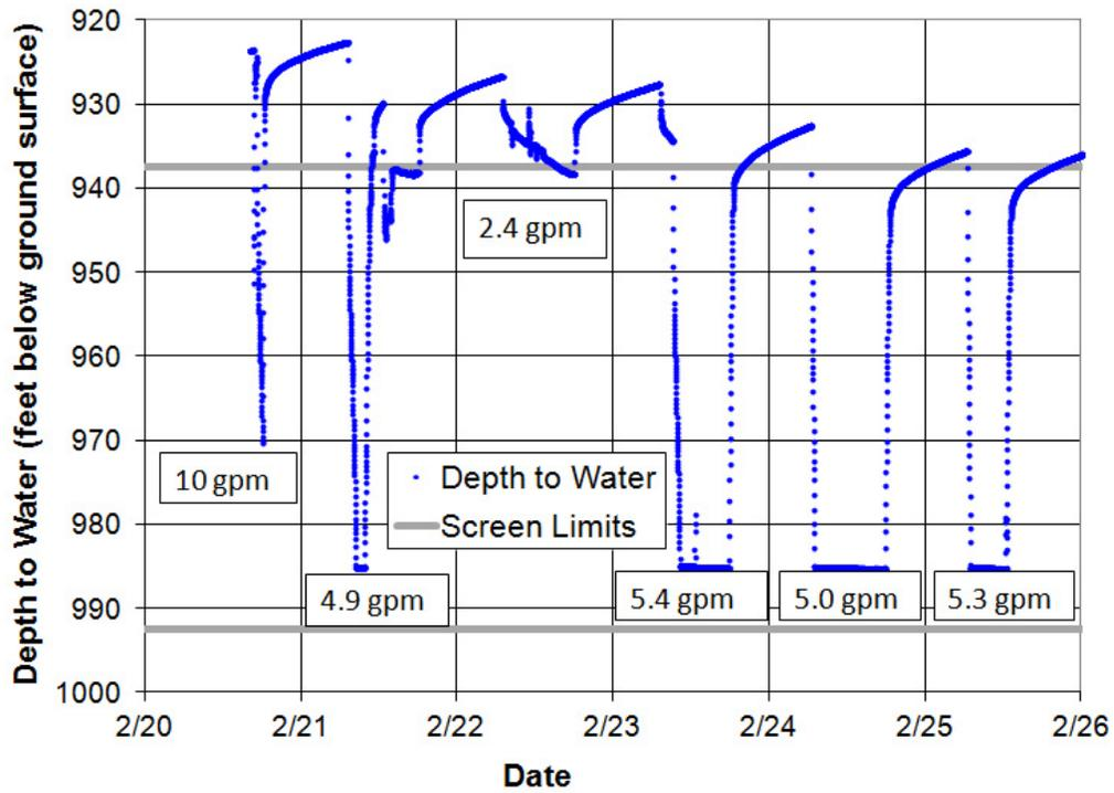
Figure F-9.3-2 Well CdV-9-1(i) screen 1 final purging—expanded scale
