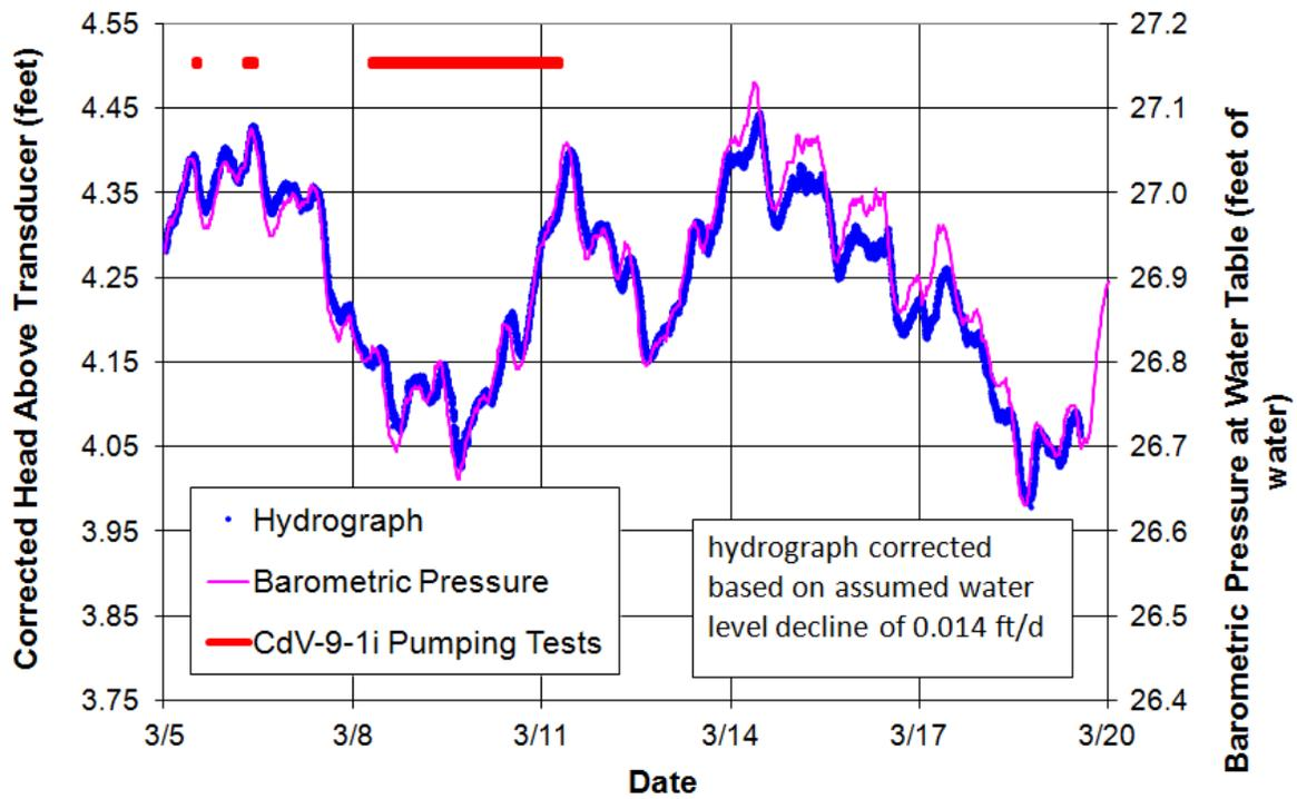
Figure F-8.0-4 Well R-63i corrected apparent hydrograph
