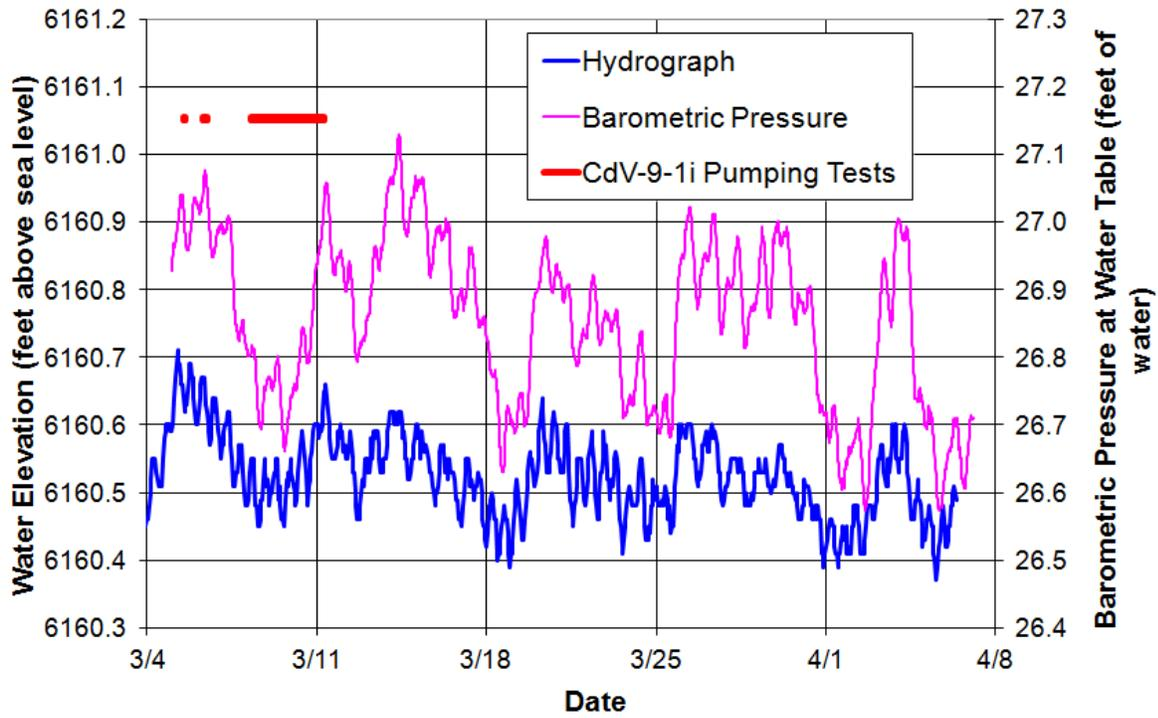
Figure F-8.0-17 Well R-25 screen 7 apparent hydrograph
