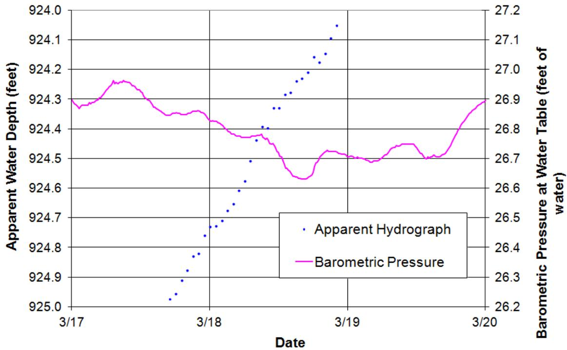
Figure F-8.0-2 Well CdV-9-1(i) apparent hydrograph—expanded scale
