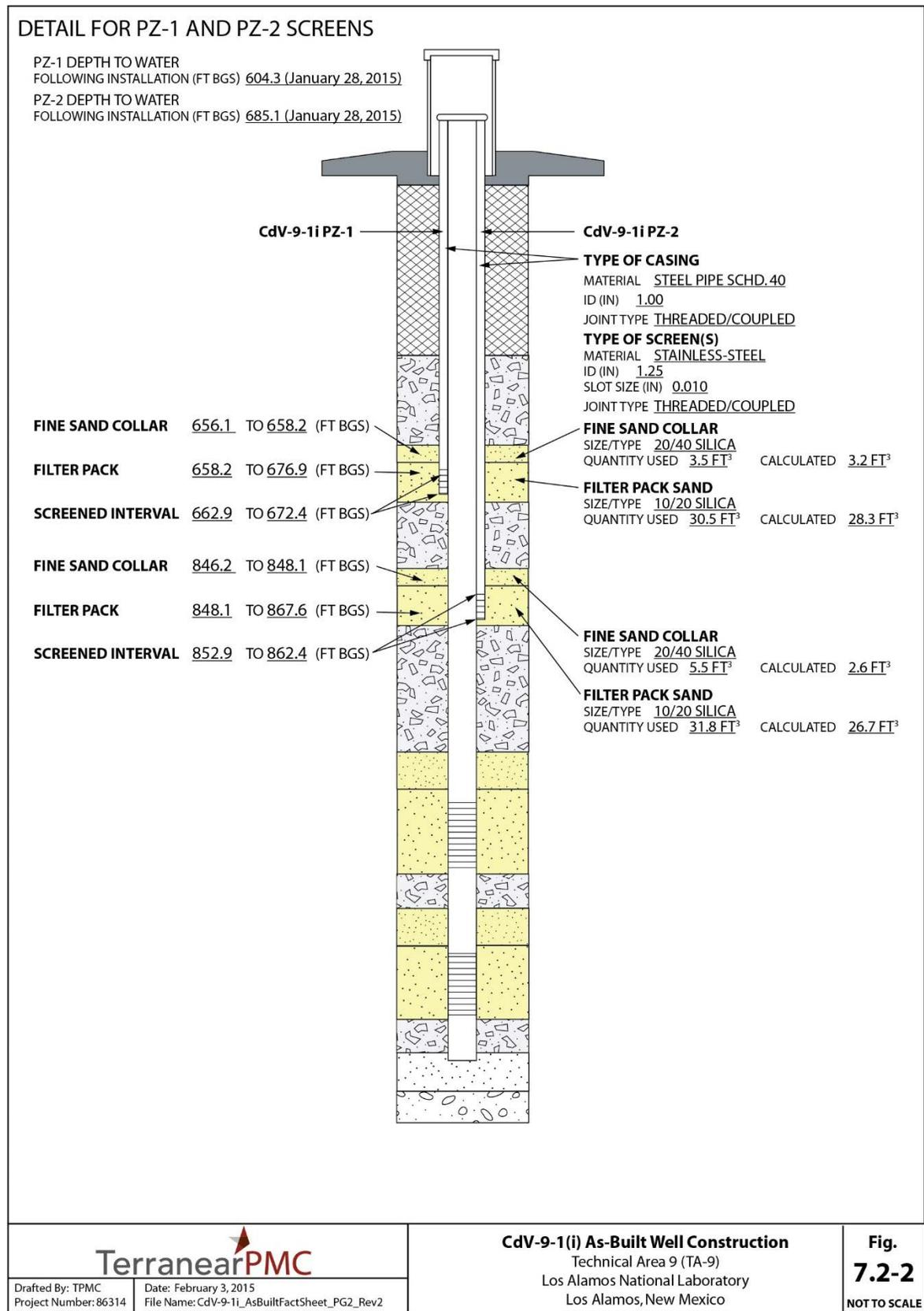
Figure 7.2-2 Monitoring well CdV-9-1(i) as-built well construction diagram
