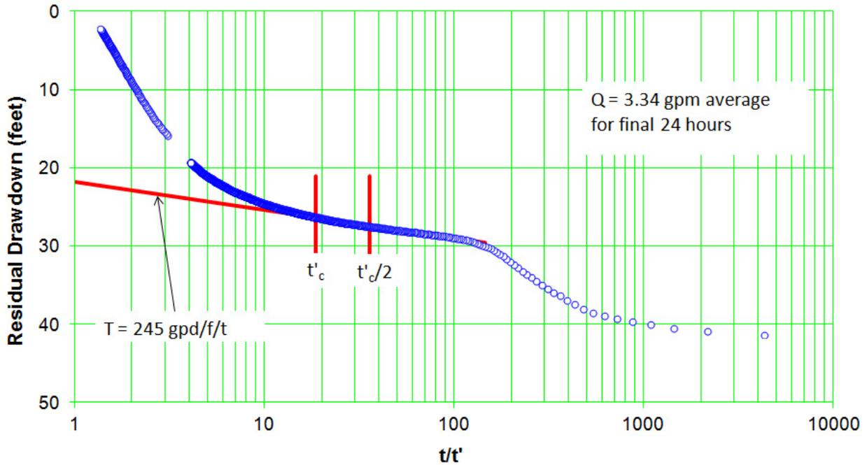
Figure F-9.2-3 Well CdV-9-1(i) screen 1 modified recovery
