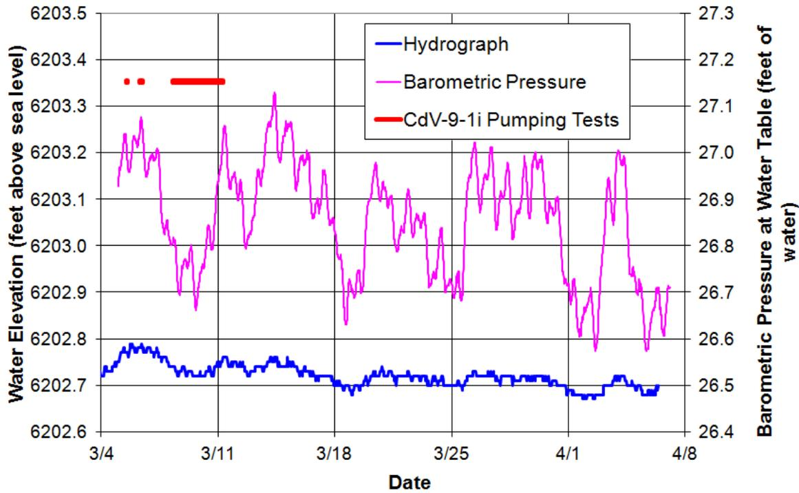
Figure F-8.0-16 Well R-25 screen 6 apparent hydrograph
