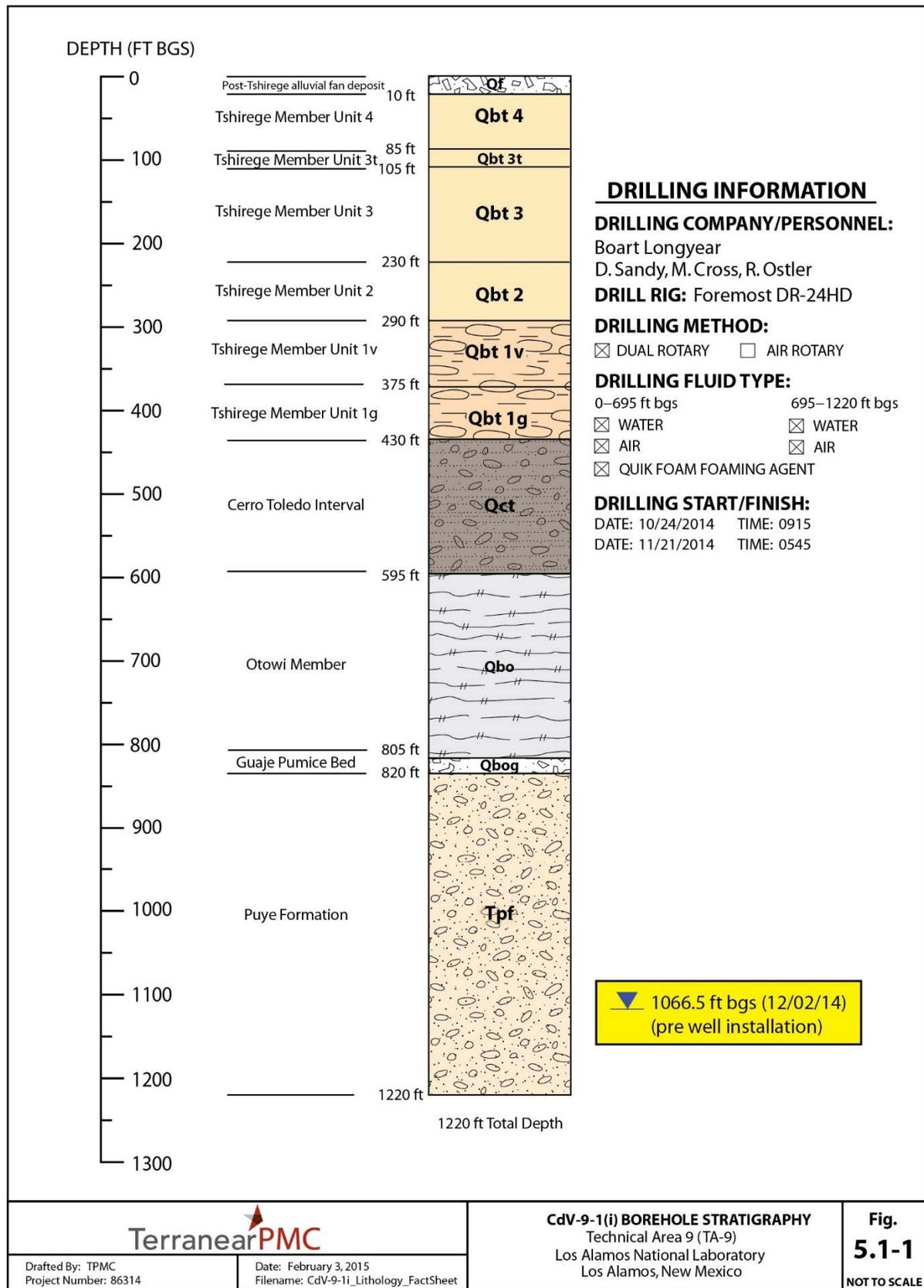
Figure 5.1-1 Monitoring well CdV-9-1(i) borehole stratigraphy
