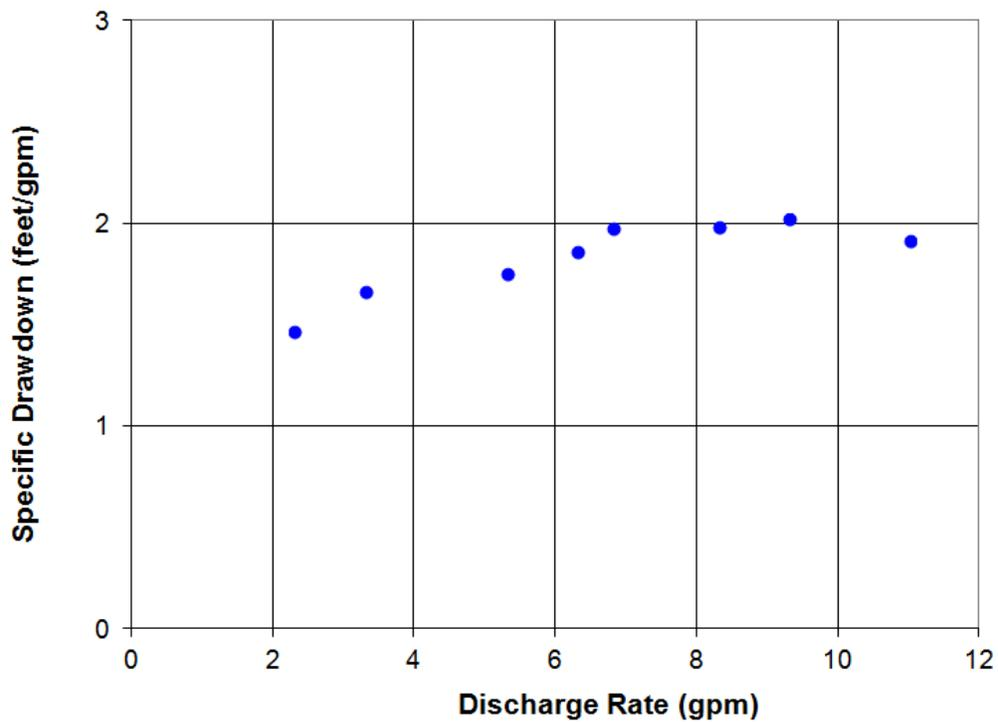
Figure F-9.1-2 Well CdV-9-1(i) screen 1 corrected specific drawdown
