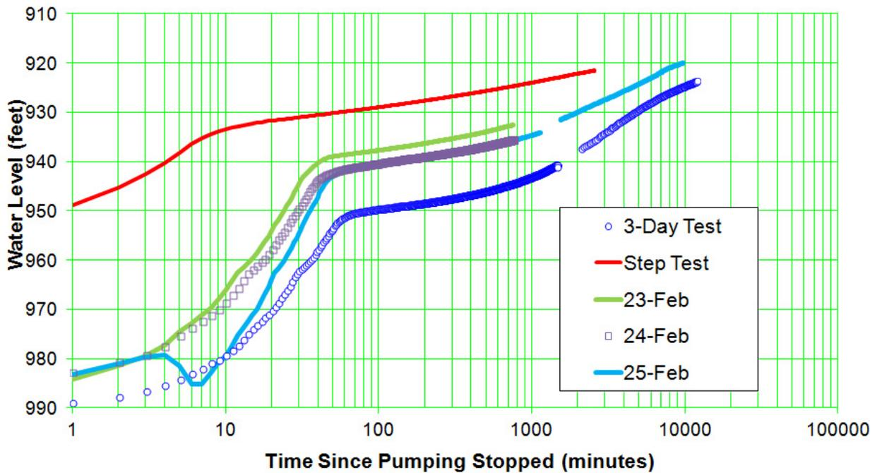
Figure F-9.3-3 Well CdV-9-1(i) screen 1 recovery for multiple tests
