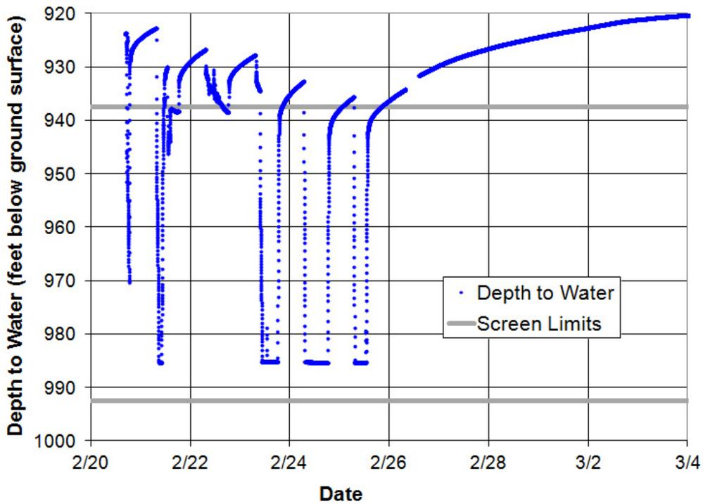
Figure F-9.3-1 Well CdV-9-1(i) screen 1 final purging
