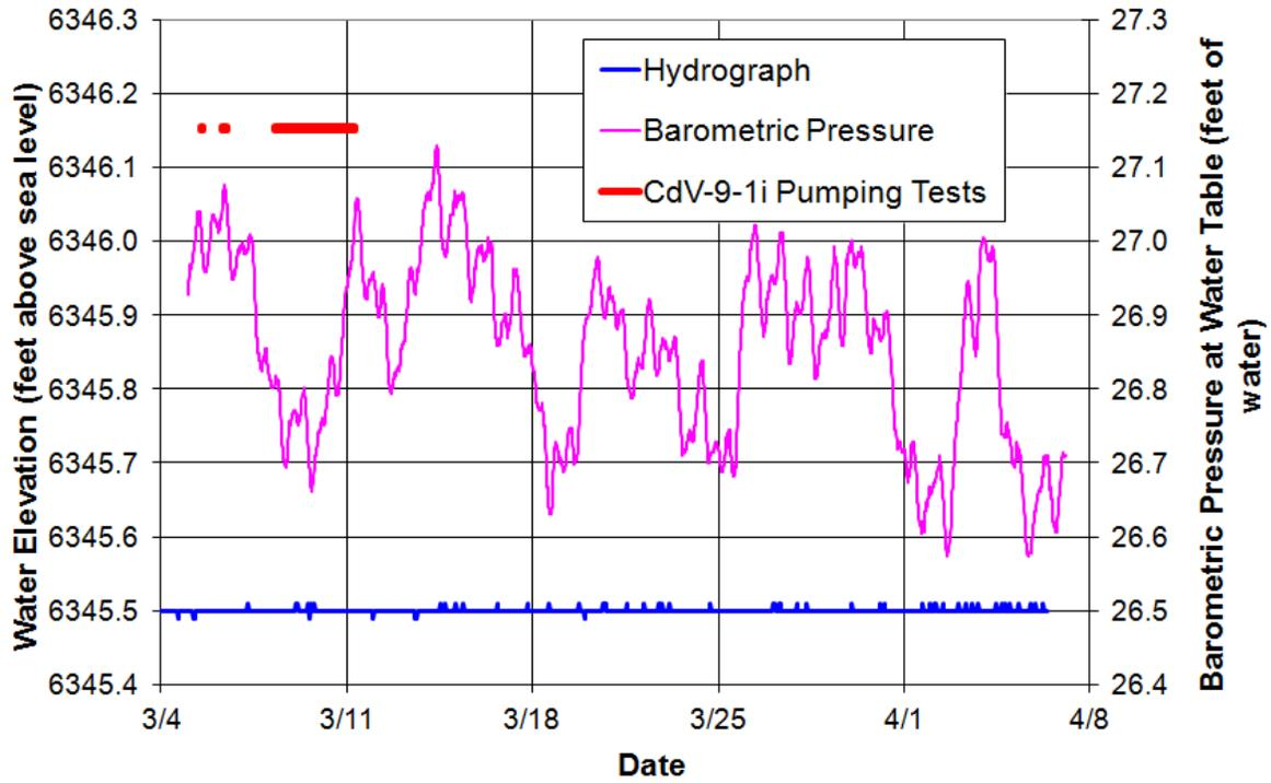
Figure F-8.0-15 Well R-25 screen 4 apparent hydrograph
