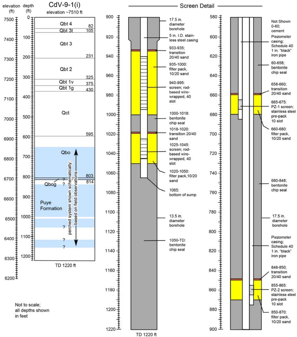
Figure 1. Proposed well design, CdV-9-1(i) (Qbt 4, 3t, 3, 2, 1v, 1g = subunits of the Tshirege Member of the Bandelier Tuff; Qct = Cerro Toledo interval; Qbo = Otowi Member of Bandelier Tuff; Qbog = Guaje Pumice Bed..
