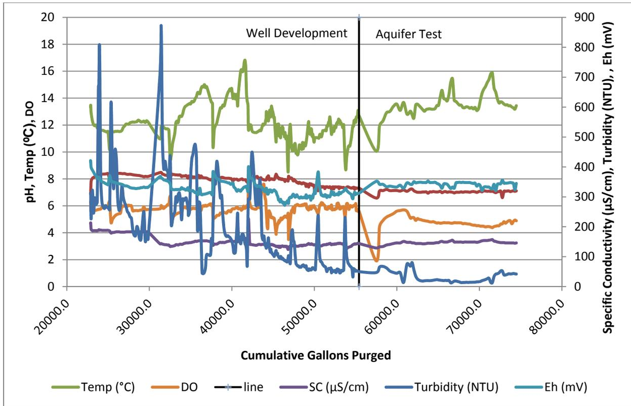
Figure B-2.2-1 Field parameters versus volume purged during CdV-9-1(i) well development and aquifer testing
