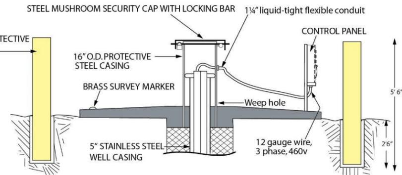
WELL HEAD DETAILS SECTION A-A'
