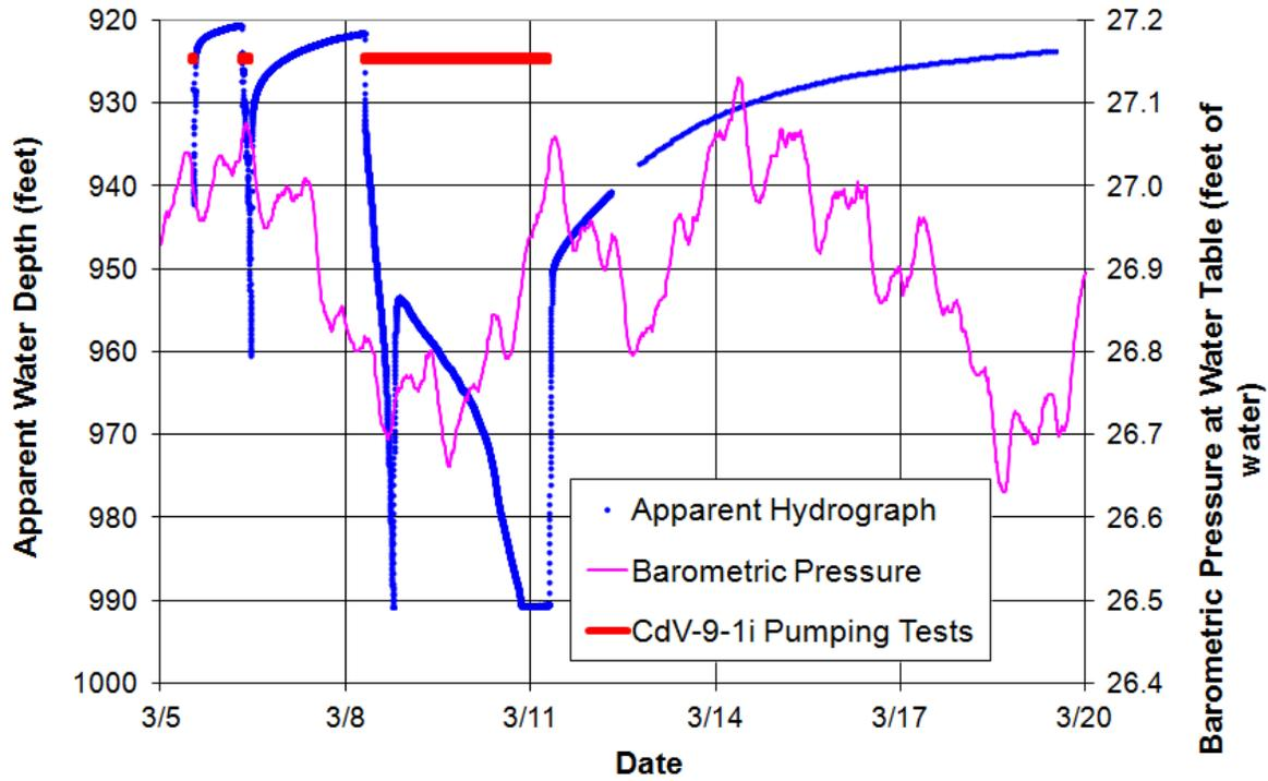
Figure F-8.0-1 Well CdV-9-1(i) apparent hydrograph and barometric pressure
