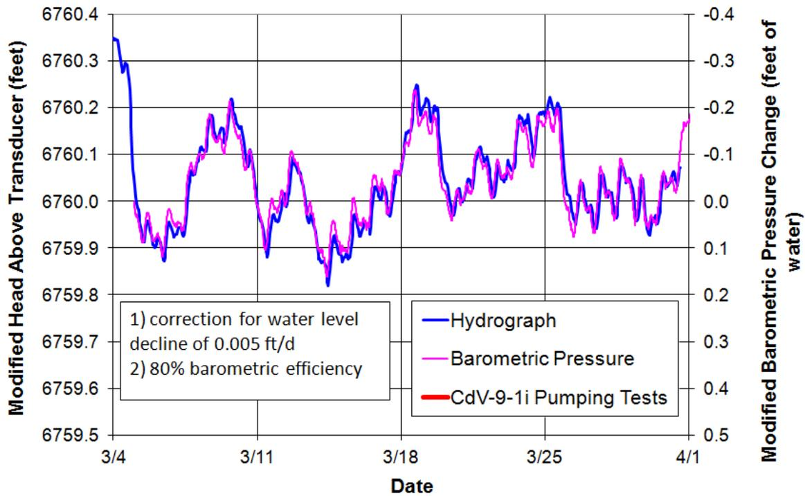
Figure F-8.0-12 Well R-25b hydrograph and barometric pressure correlation
