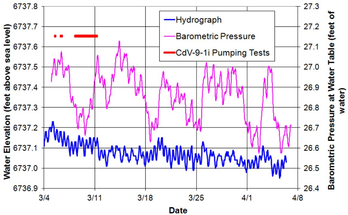
Figure F-8.0-14 Well R-25 screen 2 apparent hydrograph
