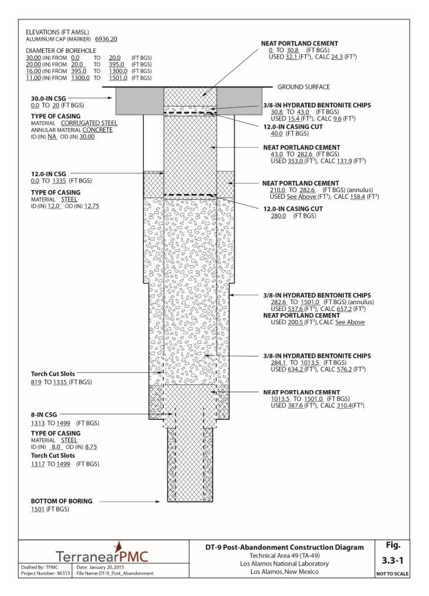
Figure 3.3-1 Test well DT-9 post-abandonment construction diagram
