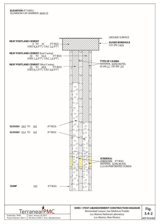
Figure 3.4-2 Test well SIMO-1 post-abandonment construction diagram
