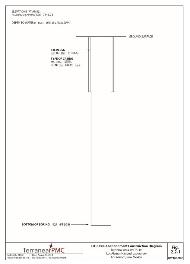
Figure 2.2-1 Test well DT-5 pre-abandonment construction diagram
