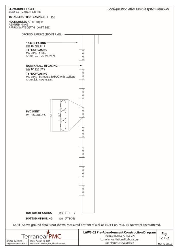
Figure 2.1-2 Well LAWS-02 pre-abandonment construction diagram
