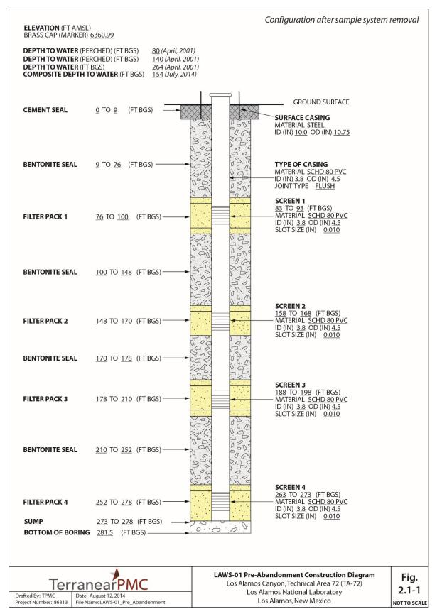
Figure 2.1-1 Well LAWS-01 pre-abandonment construction diagram
