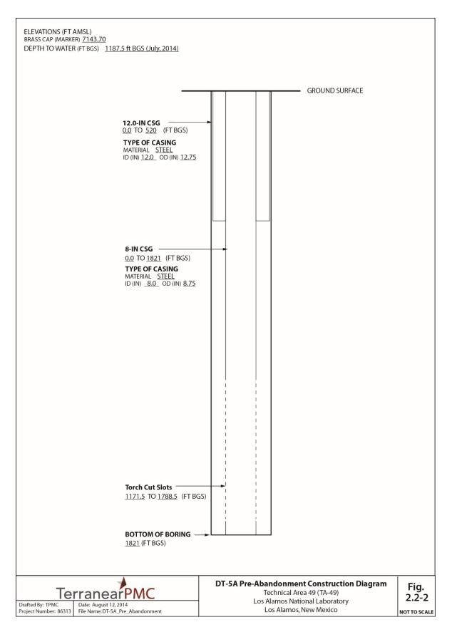
Figure 2.2-2 Test well DT-5A pre-abandonment construction diagram
