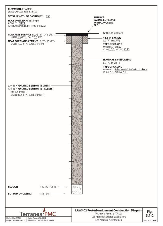
Figure 3.1-2 Well LAWS-02 post-abandonment construction diagram
