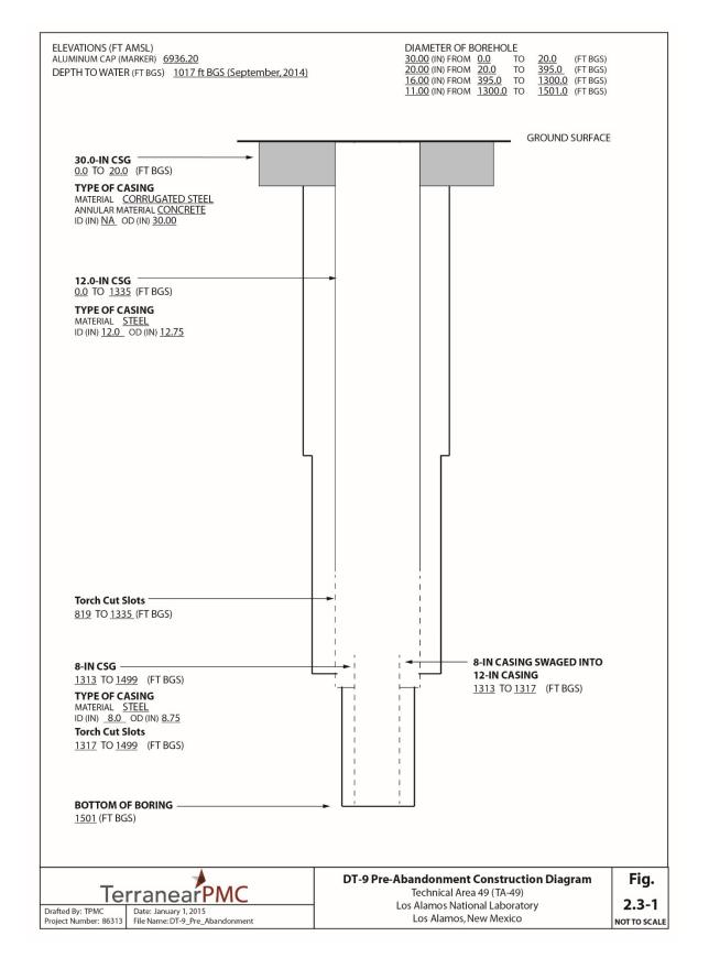
Figure 2.3-1 Test well DT-9 pre-abandonment construction diagram
