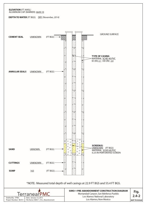
Figure 2.4-2 Test well SIMO-1 pre-abandonment construction diagram
