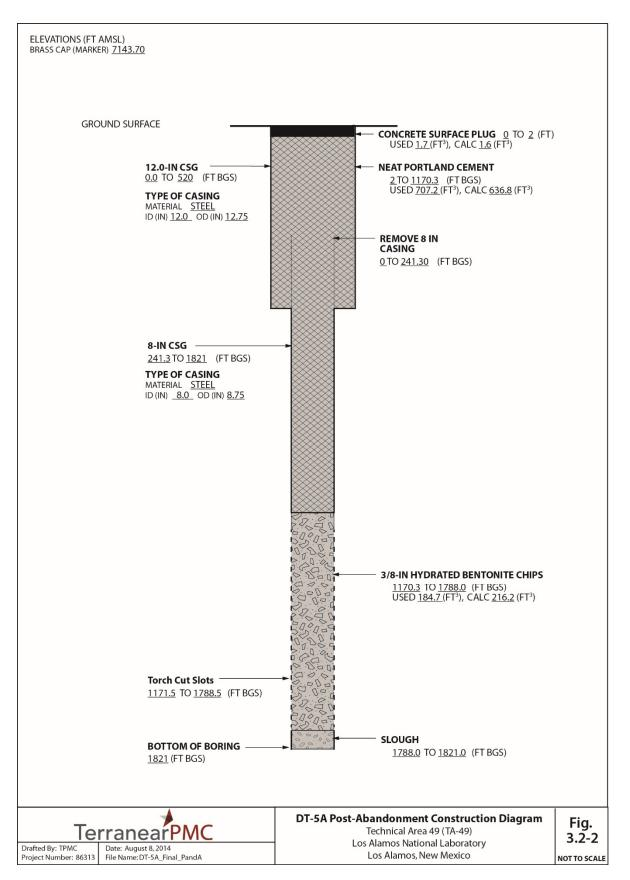
Figure 3.2-2 Test well DT-5A post-abandonment construction diagram
