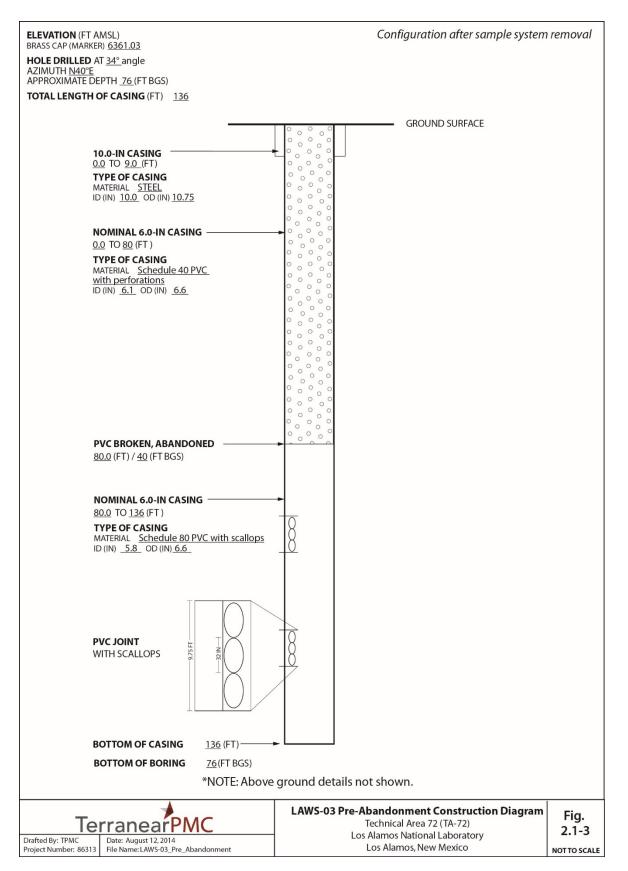
Figure 2.1-3 Well LAWS-03 pre-abandonment construction diagram
