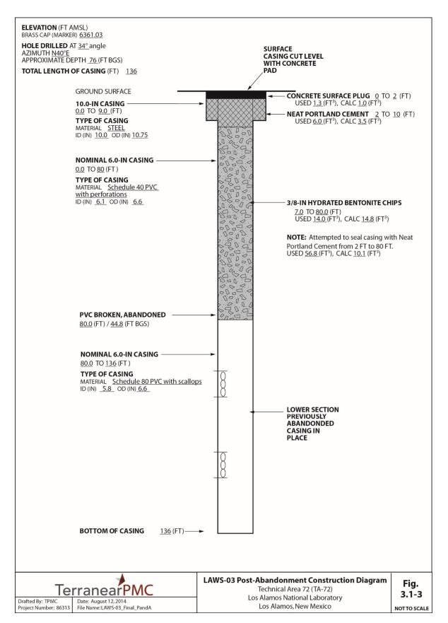
Figure 3.1-3 Well LAWS-03 post-abandonment construction diagram
