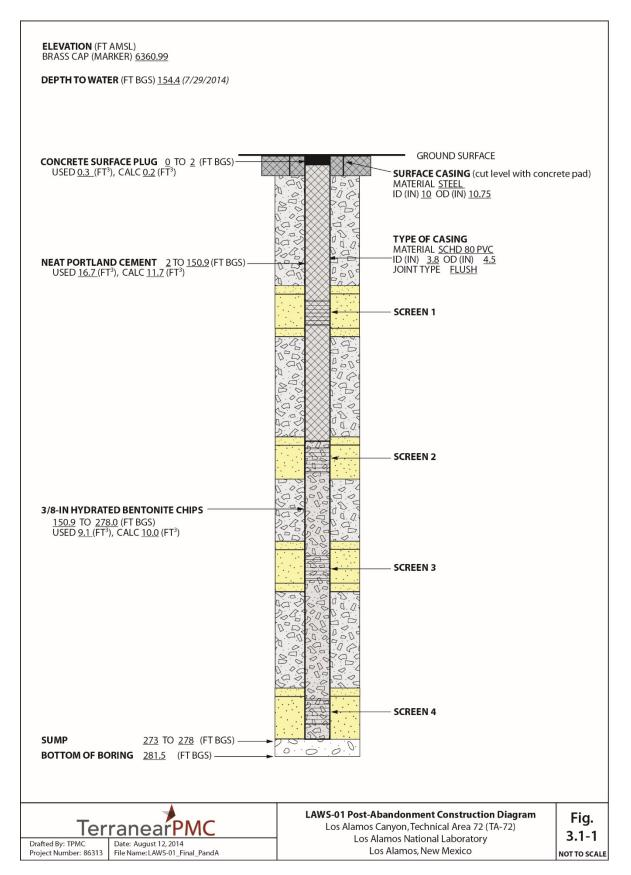
Figure 3.1-1 Well LAWS-01 post-abandonment construction diagram
