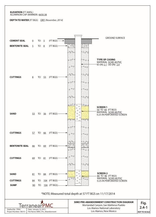
Figure 2.4-1 Test well SIMO pre-abandonment construction diagram
