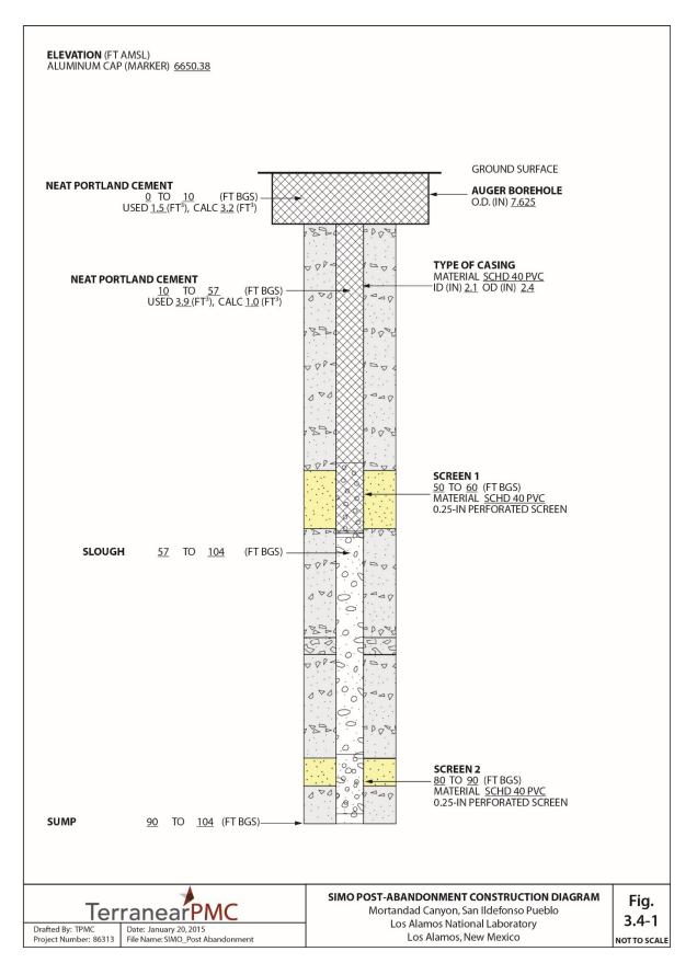
Figure 3.4-1 Test well SIMO post-abandonment construction diagram
