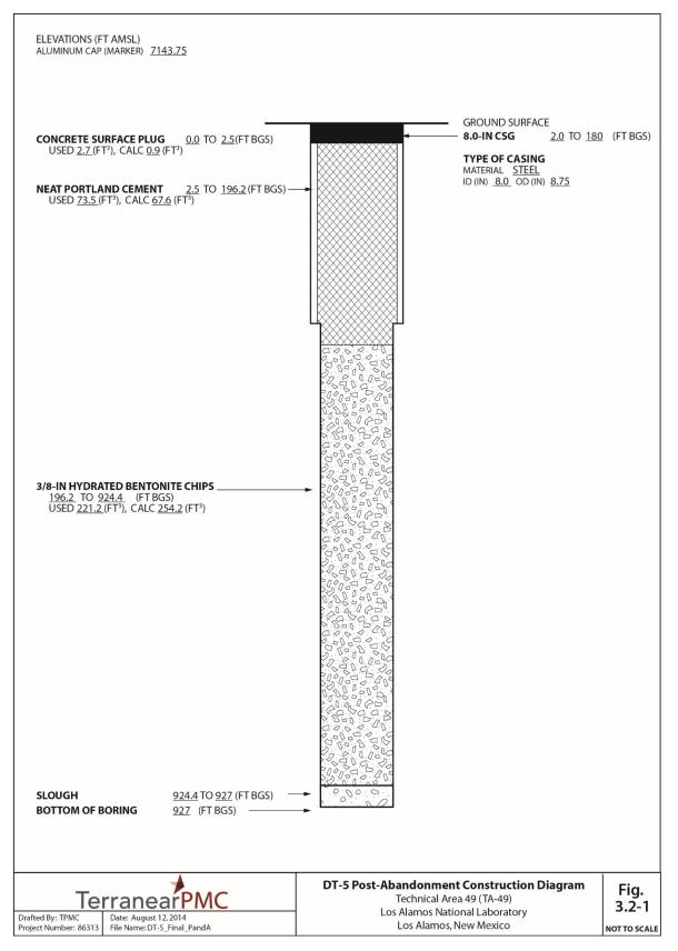
Figure 3.2-1 Test well DT-5 post-abandonment construction diagram
