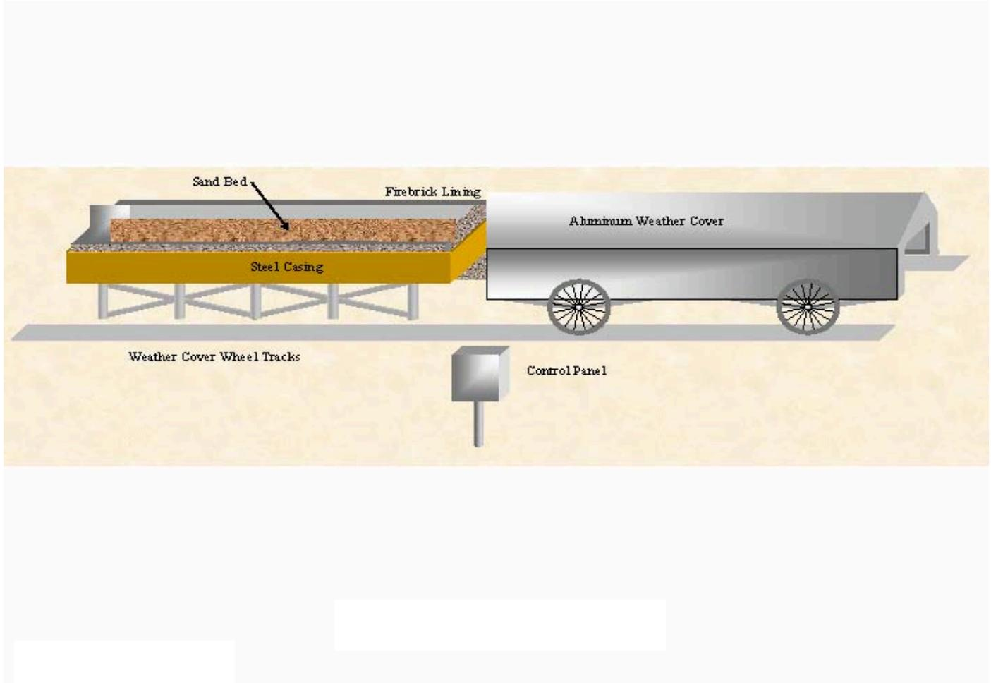
**Figure 3:** Technical Area 16-399 Open Burning Treatment Unit Configuration
