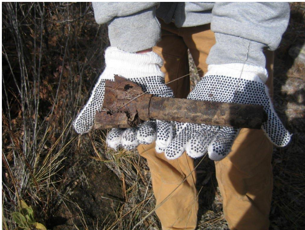
Figure 5.2-2 Fragment of 2.38-in. expended rocket motor with fin assembly found at SWMU 00-011(d) in 2013
