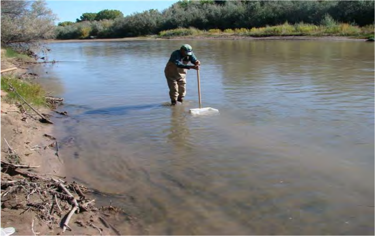
Figure 8-23 Collecting benthic macroinvertebrates (BMIs) in the Rio Grande using a kick net
