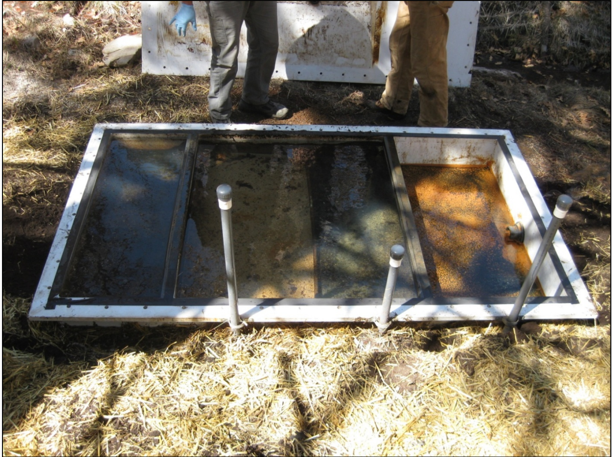
Figure 4.2-3 Equilibration of water levels inside PRB vessel
