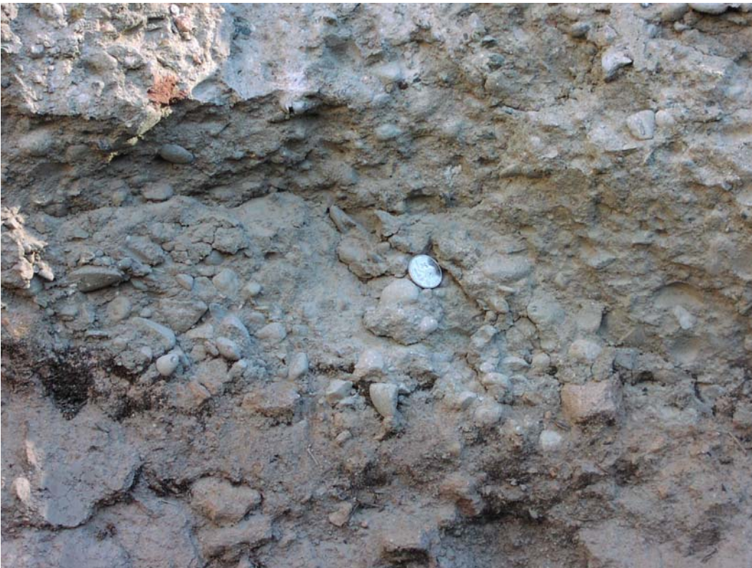
Figure 5. Close-up of RCC construction material. Quarter is placed to show scale.
